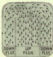
The **Oven Flue** used in all “Treasure” Base Burners is so constructed that the fire travels over the oven top, down the back and under the oven at both sides to the base of the stove, and returns up the flue in the centre. You will note by this that the fire travels around the oven twice before entering the chimney, economizing to the extent of about 40%, and baking equal to a cook stove.
