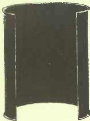
“Treasure Oak” Bodies are made of one piece Heavy Superior Cold Rolled Steel and Flanged Top and Bottom. In mounting, the body is forced over a flange on top of Fire-Pot into cement filled cup joint. Body flange is then turned, and over this Deflector Ring is bolted, making an absolutely air-tight joint, which cannot open or leak.
