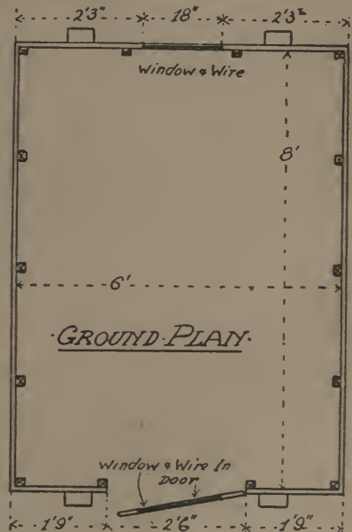
Ground plan of Colony House for growing stock.
