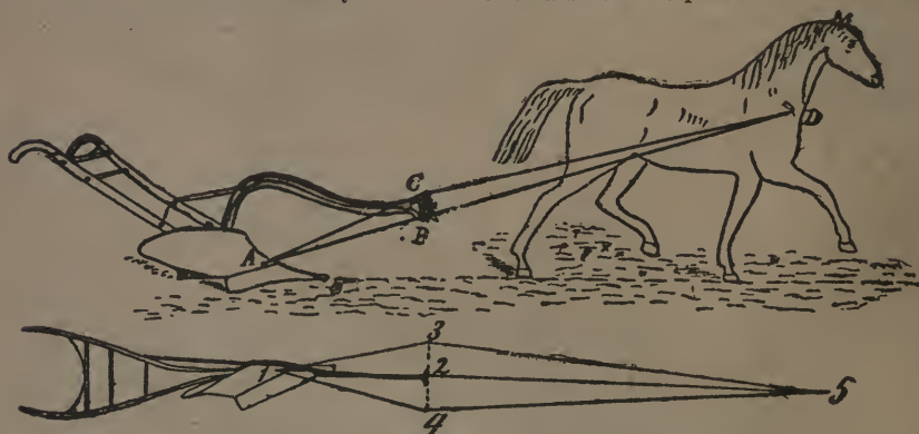
Direction of the line of draft for plows.
