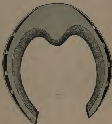
Toe weight to increase length of stride. The weight is properly placed, but the nails should go further forward.
