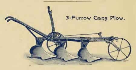
Built after the model of our No. 2 Gang, having extra high Standards, large Mouldboards. Frame entirely of Steel, Axles with long Chilled Bearings. Turns three 9-inch furrows. Used largely in Manitoba, but adapted to any section in Ontario. Made with one or two levers as desired.
