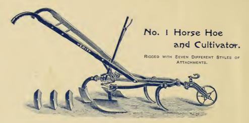
Furnished with 1 Lever, 5 Standards, 5 Diamond or Oval Points, 2 Short Hillers, and 1 Shovel Blade. Long Hillers furnished, if desired. Made of best quality Steel. Strong enough to stand immense strain. Light and easy to handle. By use of Lever the width can be instantly and easily changed while in motion. Standards are hollow Steel, pressed to a shape that will stand the greatest strain, and are guaranteed not to bend. All blades are of the highest quality tempered steel.
