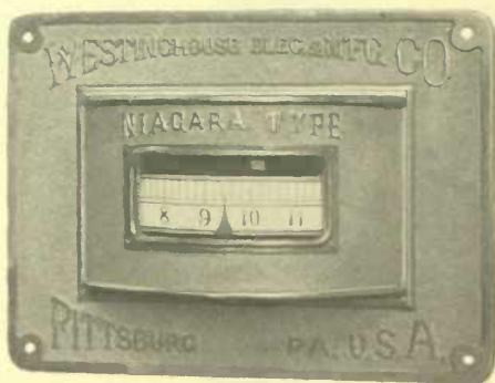
AN ALTERNATING CURRENT AMMETER, NIAGARA TYPE.
