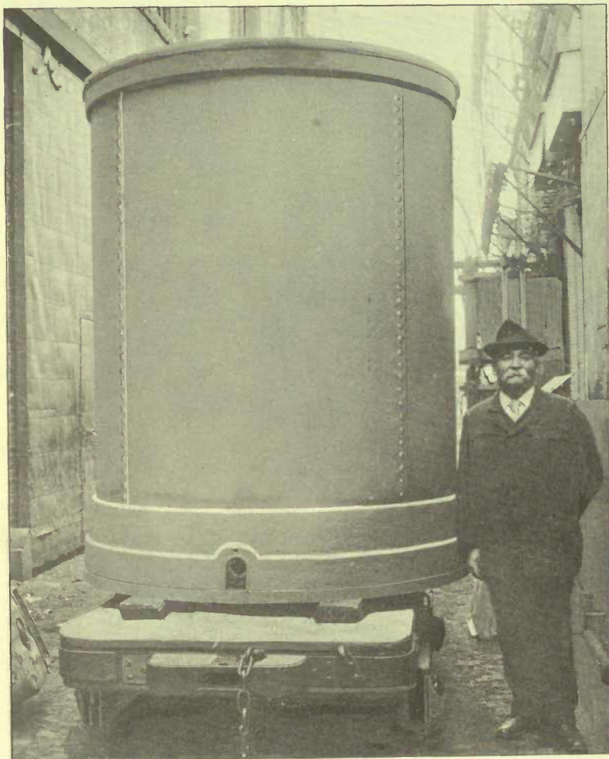
ONE THOUSAND HORSE-POWER STATIC TRANSFORMER AT THE WORKS OF THE CARBORUNDUM COMPANY. BUILT BY THE GENERAL ELECTRIC CO. NEW YORK.
