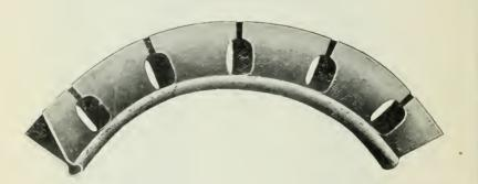
Pedlar's "Perfect" Plasterers' Corner Bead as used on segment arches. This corner bead can be curved to any size radius by cutting with a pair of tinner's snips as shown in this illustration. Outlines a true circle to guide the plasterer.
