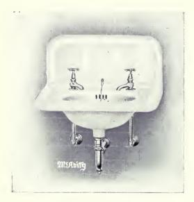
McAvity's Porcelain Enameled Cast Iron Lavatory, with Slab, Oval Bowl with Centre Outlet, Overflow and Back in One Piece, supported on concealed Wall Hanger; fitted with "Royal B" Compression Faucets; "Royal Angle" Supplies to Wall, and 1¼" "Royal" P. Trap. with Chain and Stopper.
