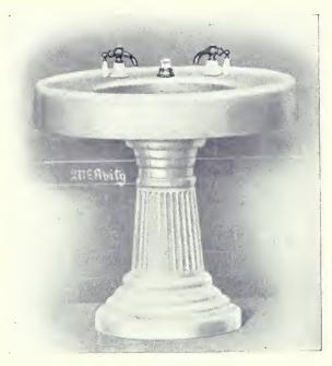
McAvity's Porcelain Enameled Cast Iron Pedestal Lavatory, with Slab, D Shaped Bowl, with Rear Outlet and Apron in One Piece, supported on Porcelain Enameled Fluted Pedestal; fitted with "Royal" Fuller Design Faucets, with China Base and China Lever handles; ½" I.P. Size "Royal Anglo" Supplies, with China Indexed Stop Valves and "Royal" Bi-Transit Waste, with 1½" Bag Trap to Wall.
