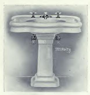
Pedestal Lavatory, with Slab, Oval Bowl with Rear Outlet and Apron, in One Piece, supported on Square Pedestal and Enameled all over; fitted with "Royal Lorna" Compression Combination Supply and Waste Fitting, with China Index Handles on Faucets, and China Knob on Waste; ½" I.P. Size "Royal Anglo" Supplies with Indexed Stop Valves on Supplies and 1½" "Royal" P. Trap to Wall.
