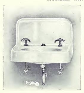
McAvity's Porcelain Enameled Cast Iron Lavatory, with Slab, "D" Shaped Bowl with Rear Outlet, Back and Apron in One Piece, supported on concealed Wall Hanger; fitted with "Royal Fuller" Design Faucets; ½" I.P. Size "Royal Anglo" Supplies, with Indexed Stop Valves; "Royal" Bi-Transit Waste, with 1½" "Royal" Bag Trap to Wall.
