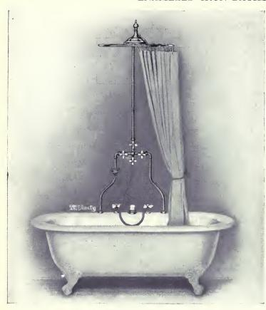
McAvity's Porcelain Enameled Iron Bath, with 4¾" Roll Rim; fitted with Royal "Olympic" Bottom Bell Supply and Waste Fitting; ¾" Supply Pipes, with unions at Floor; China Indexed Cross Handle Compression Valves, and China Knob on Waste; Nickel Plated 8" Shower Head Combination, Shampoo with Rubber Hose and Sprinkler; China Indexed Cross Handle Controlling Valves; Ring and Duck Curtain.
