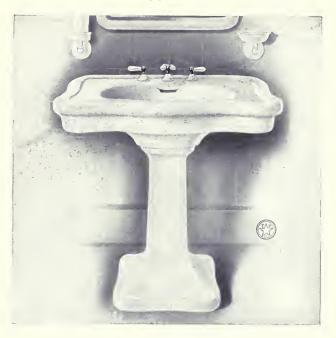
McAvity's Solid Vitreous China Serpentine Design All-Roll Rim Lavatory. Oval Bowl, with Integral Spout and Mixing Chamber, with Anti-Splash Rim, supported on plain Square Pedestal; fitted with "Royal" China Lever Handle Quick-Opening Compression and China Cross Handle Pop-up Waste Combination; "Royal Angle" Supplies, with Indexed Stop Valves and  $1\frac{1}{4}$ " Royal Nickel Plated Trap to Wall.
