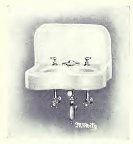
McAvity's Porcelain Enameled Cast Iron Lavatory with Slab, "Kidney" Design Bowl with Rear Outlet, Back and Apron in One Piece; fitted with "Royal Neva" Fuller Design Combination Supply and Waste Fitting, with 1½" "Royal" Bag Trap to Wall; ½" I.P. Size "Royal Anglo" Supplies, with Indexed Stop Valves.
