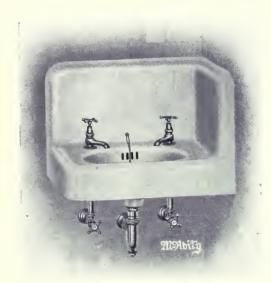
McAvity's Porcelain Enameled Cast Iron Lavatory, for Right Hand Corner, with Slab, Oval Bowl with Rear Outlet, Overflow, Back, Right Hand End Piece and Apron in One Piece, supported on concealed Wall Hanger; fitted with "Royal OK" China Indexed Compression Faucets; "Royal Anglo" ½" I.P. Size Supplies, with China Indexed Stop Valves, Chain and Stopper; 1½" "Royal" P, Trap to Wall.
