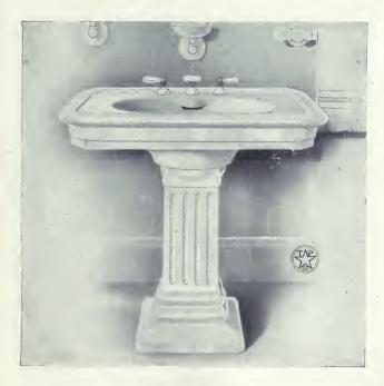
McAvity's Solid Vitreous China Square Design All-Roll Rim Pedestal Lavatory. Oval Bowl, with Integral China Spout and Mixing Chamber, with Anti-Splash Rim, supported on Fluted Square Pedestal; fitted with Royal-China Lever Handle, Quick Opening Compression and China Cross Handle Pop-up Waste Combination; "Royal Anglo" Supplies, with Indexed Stop Valves and 1½" Royal Nickel Plated Trap to Wall.
