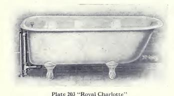
McAvity's Porcelain Enameled Cast Iron Bath with 21/2" Roll Rim, Wide Flat Bottom Design; fitted with "Royal Presto" Quick Opening Bath Faucets; 5%" O.D. "Royal" Nickel Plated Bent Supplies and "World" Combined Waste and Overflow.
