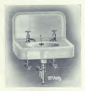
McAvity's Porcelain Enameled Cast Iron Lavatory, with Slab, Oval Bowl with Centre Outlet, Overflow, Back and Apron in One Piece, supported on concealed Wall Hangers; fitted with "Royal World" Compression Faucets; ½" I.P. Size "Royal Anglo" Supplies, and "Royal" P. Trap to Wall.
