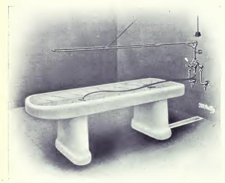
Washing Table for Hospitals, with Pedestals, in best quality Excelsior White Porcelain, with Nickel Plated Fittings, comprising 34" Hot and Cold Bibbs, with Stays to Wall, Body Spray with Hinges, Pulley, Balance Weight and Chain for swinging up to the wall when not in use, Hand Spray with Rubber Tube, 2" Outlet Grating and Down Pipe to Discharge into Channel.
