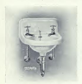
McAvity's Porcelain Enameled Cast Iron Lavatory, with Slab, Round Bowl with Centre Outlet, Overflow and Back in One Piece, supported on concealed Hangers; fitted with "Royal OK" Faucets, with China Indexed Handles; 5%" O.D. "Royal Angle" Supplies, 1¼" "Royal" P. Trap, with Chain and Stopper.
