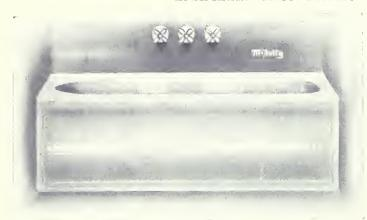
McAvity's Porcelain Enameled Cast Iron Recess Baths, with Centre Outlet, and 4" Roll Rim; fitted with Royal "Utopia" Bottom Bell Supply and Waste Combination, concealed in Wall; 34" I.P. Size Brass Supplies; Compression Valves with Indexed China Cross Handles, and Indexed China Cross Handle Waste, with China Escutcheons.
