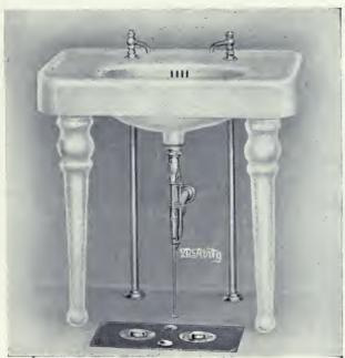
in One Piece, supported on Porcelain Enameled Legs; fitted with "Royal Trident" Combination Floor Plate, with Self-Closing Foot-Operated Hot and Cold Supplies, and Foot Operated Waste, with 1½" "Royal" Trap, as illustrated. The Valves are below floor. If desired the valve motion can be furnished above floor.
