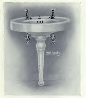
McAvity's Porcelain Enameled Cast Iron Pedestal Lavatory, with Slab, "D" Shaped Bowl with Rear Outlet, Overflow and Apron in one Piece, supported on Enameled Pedestal Leg and Wall Supports, enameled all over; fitted with "Royal World" Compression Faucets; 1/2" I.P. Size "Royal Anglo" Supplies, with Indexed Stop Valves; 11/2" Royal P. Trap to Wall with Chain and Stopper.
