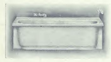
McAvity's Porcelain Enameled Cast Iron Recess Bath, with 3" Roll Rim; fitted with "Royal Utopia" Bottom Bell Supply and Waste Combination; 34" I.P. Size Supplies concealed in Wall; Compression Valves with Indexed China Cross Handles, and Indexed China Cross Handle Waste with China Escutcheons.
