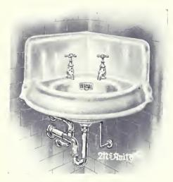
McAvity's Porcelain Enameled Cast Iron Corner Lavatory, with Slab, "D" Shaped Bowl with Rear Outlet, Overflow, Back and Apron in One Piece, supported on concealed Wall Hangers; fitted with "Royal OK" China Indexed Faucets; 5%" O.D. "Royal Angle" Supplies, and 1¼" "Royal" P. Trap with Chain and Stopper.
