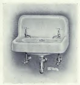
McAvity's Porcelain Enameled Cast Iron Lavatory, with Slab, "D" Shaped Bowl with Rear Outlet, Back and Apron in One Piece, supported on concealed Hangers; fitted with "Royal Swan" Compression Faucets; 5%" O.D. "Royal Anglo" Supplies with Indexed Stop Valves; 1½" "Royal" P. Trap to Wall, with Chain and Stopper.
