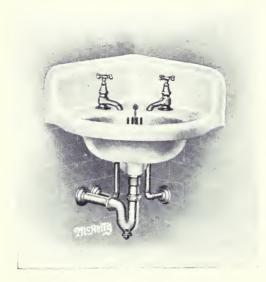
McAvity's Porcelain Enameled Cast Iron Corner Lavatory, with Slab, Round Bowl with Centre Outlet, Overflow and Back in one Piece, supported on concealed Wall Hangers; fitted with "Royal B" China Indexed Faucets; 5%" O.D. "Royal Angle" Supplies and 1½" "Royal" P. Trapwith Chain and Stopper.
