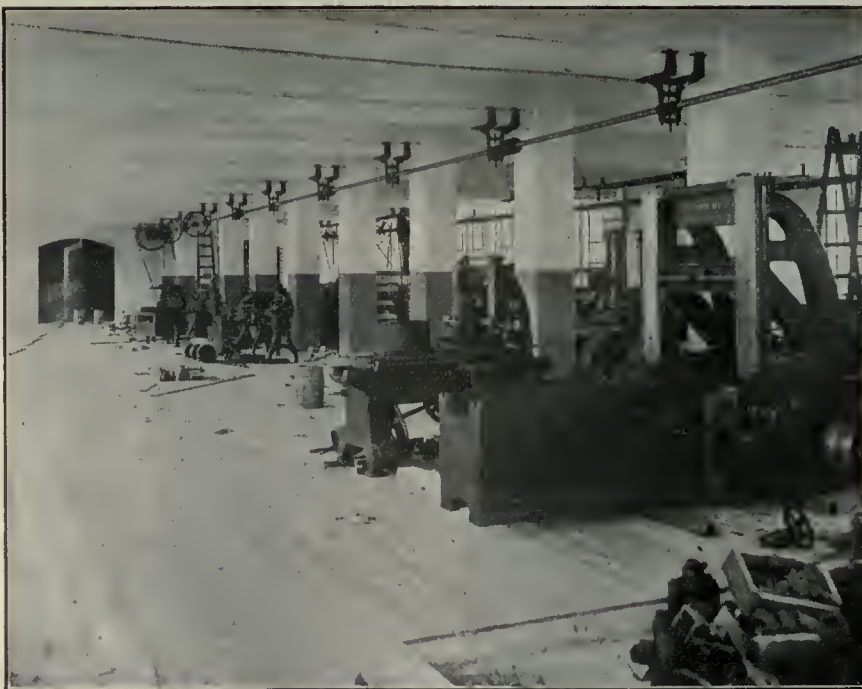
FIG. 2. LINE SHAFTING INSTALLATION IN MACHINE SHOP.
