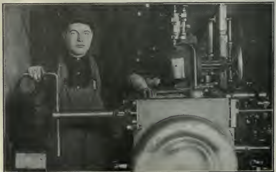
BORING OUT CORLISS VALVE SEAT IN PLACE.
