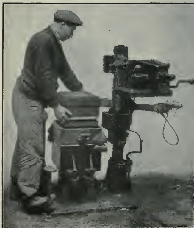
FIG. 8. REMOVING THE COMPLETED MOTTE AFTER IT HAS BEEN PUSHED OUT OF THE FLASK.
