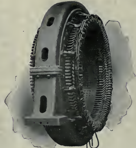
SHOWING METHOD OF SLIDING STATOR TO ONE SIDE.
