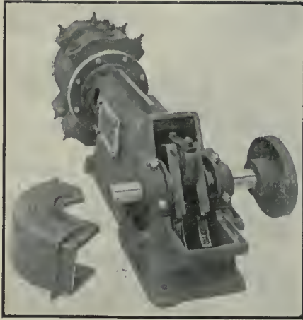
FIG. 4. SINGLE ENCLOSED FRAME, POWER DRIVEN AIR COMPRESSOR WITH FRAME CAP REMOVED.
