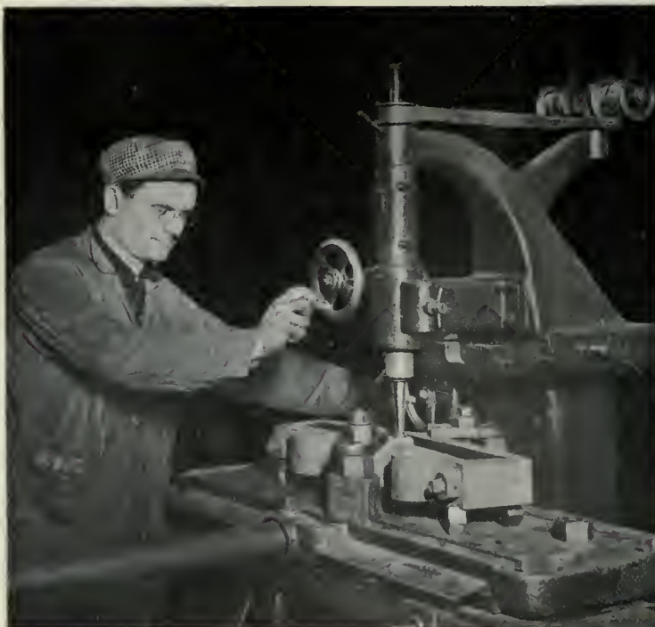
GRINDING A LINK ON A HAMMET RADIAL GRINDER.
