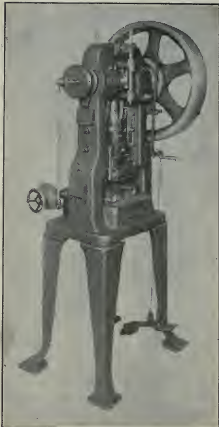
FIG. 4. SPECIAL DOUBLE ACTING SINGLE ACTING CAM PRESS.
