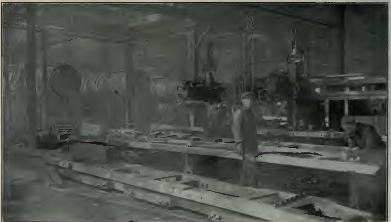
DRILLING AND FITTING LOCOMOTIVE FRAMES. THESE ARE DRILLED IN BATCHES OF FOUR AT A TIME.
