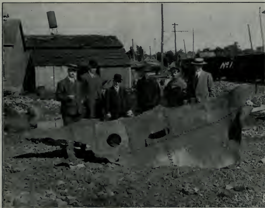
FIG. 1. TOP HALF OF BOILER SHELL BLOWN A DISTANCE OF 350 FEET.
