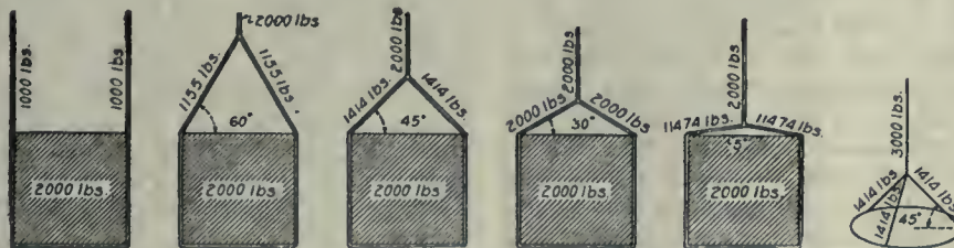
FIGS. 1 TO 6. ILLUSTRATING THE OBLIQUITY OF SLINGS.
