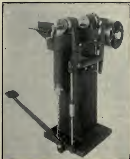
COPPER COIL FORMING MACHINE.
