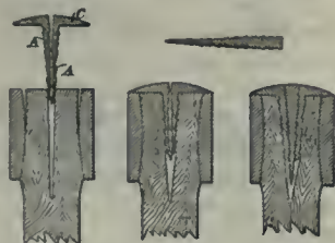
FIGS. 1, 2, 3, 4. EXPANDING WEDGE FOR HAMMER HEADS, ETC.
