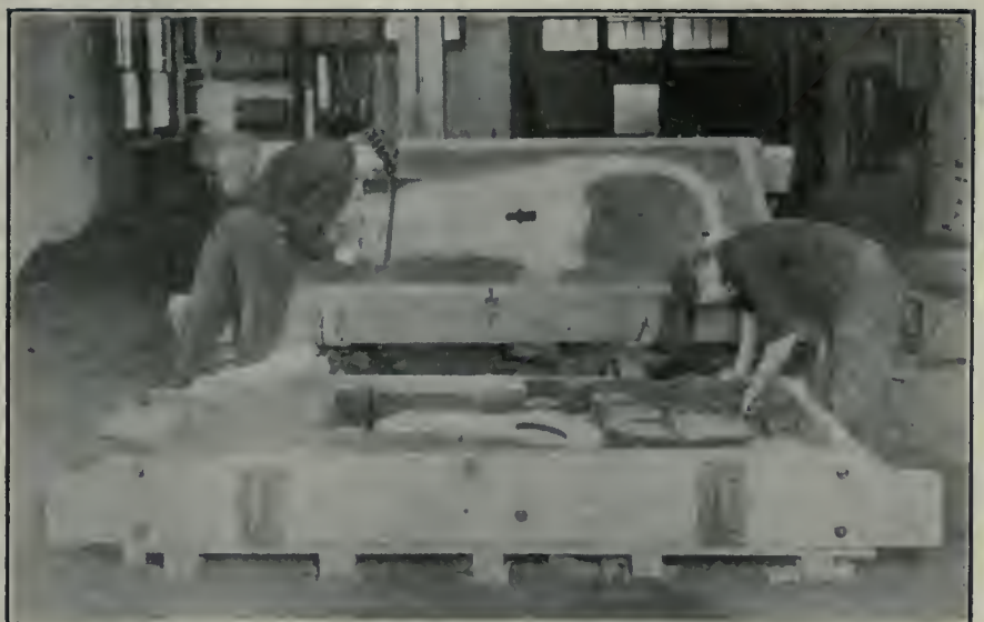
FINISHING A GREEN SAND MOLD FOR A BAND SAW FRAME. MOLD COMPLETE AND READY FOR POURING REPRESENTS ONE DAY'S WORK OF TWO STUDENTS.
