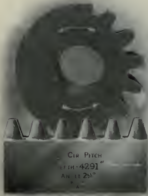
FIG. 4. RACK AND GEAR PRINCIPLE OF CUTTER OPERATION.
