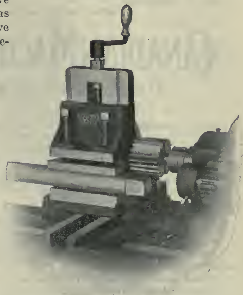
FIG. 3. SQUARING A STEEL SHAFT.
