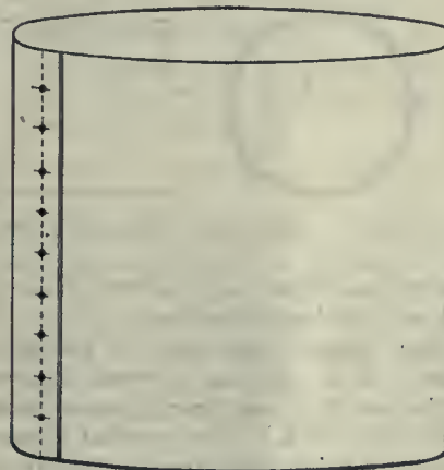
FIG. 1. NO. 22 GAUGE SHEET IRON CYLINDER.
