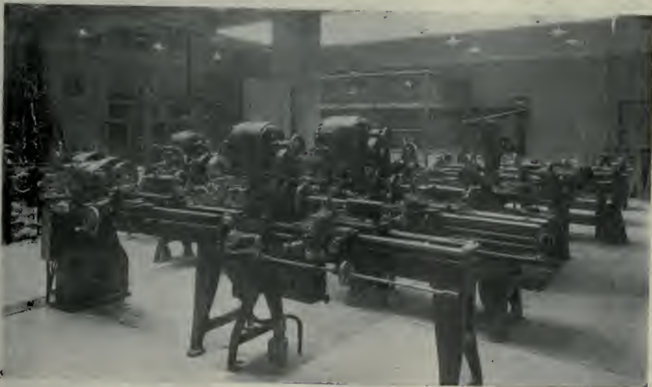
DEPARTMENT OF SHOPWORK. GROUP OF MOTOR-DRIVEN TOOL-ROOM LATHES IN MACHINE SHOP.
