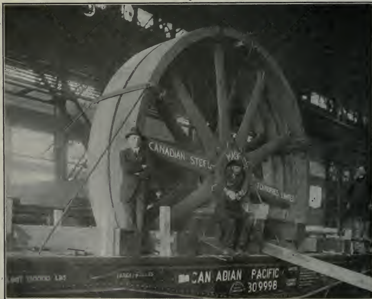
FIG. 5.—LARGE STEEL CASTING FOR ELECTRICAL MACHINERY. WEIGHT 19 TONS.
