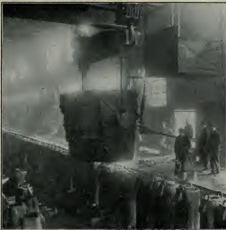
"TEEMING" THE MOLTEN STEEL INTO INGOT MOULDS.
