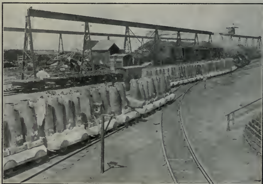
TRAIN OF INGOT Moulds EN ROUTE TO ROLLING MILL.
