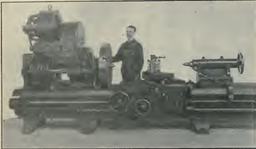
FIG. 16. 30-IN. ENGINE LATHE FOR GROOVING AND BAND TURNING.
