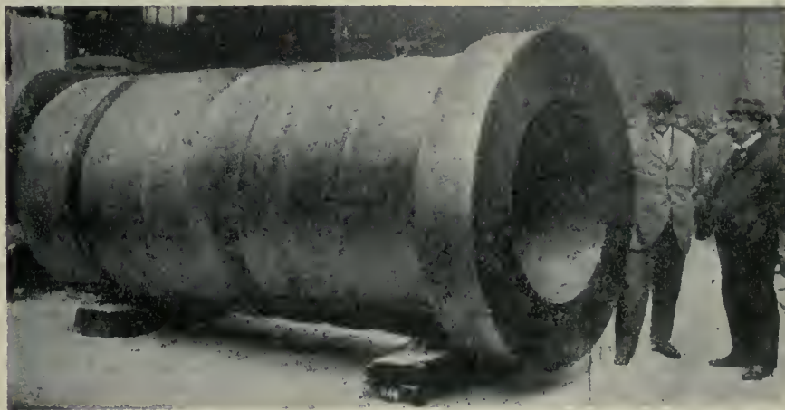
FIG. 5. AFTER ROUGH TURNING, FORGED AND EXPANDED HYDRAULIC CYLINDER AFTER ROUGH TURNING.
