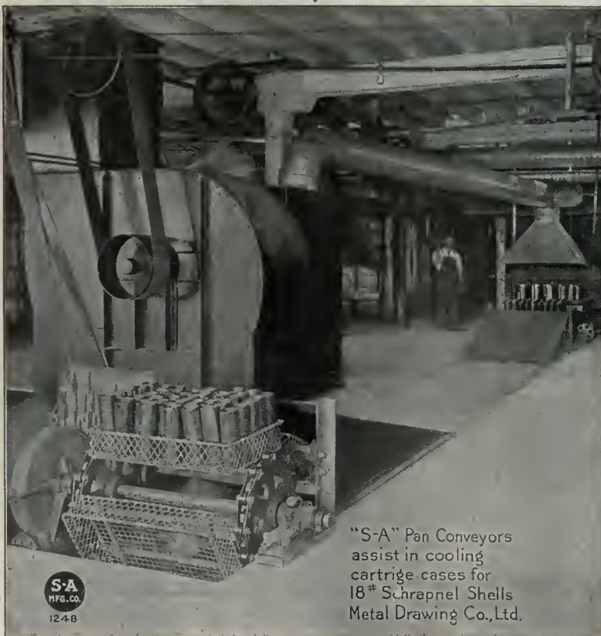
FIG. 2. DISCHARGE END OF CONVEYOR SHOWING CARTRIDGE CASES IN WIRE BASKET FOR REMOVAL TO PICKLING TANKS.
