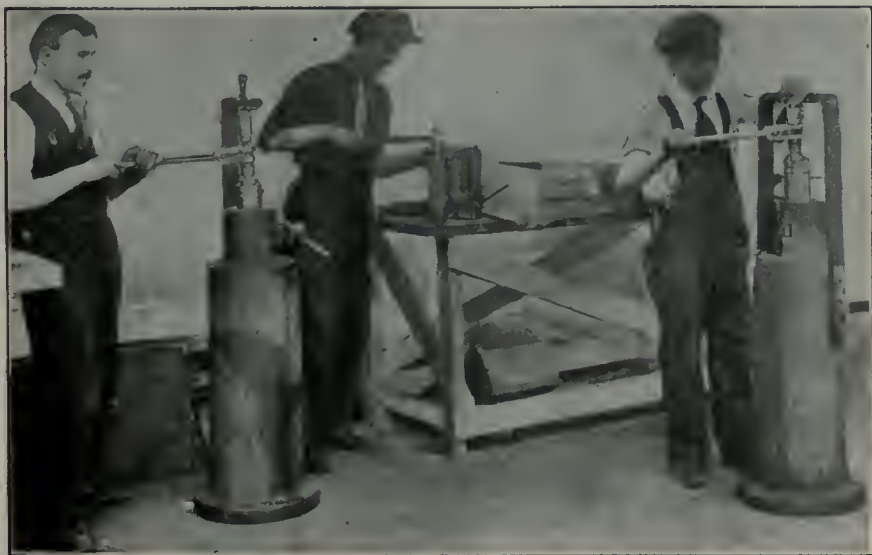
FIG. 19. SCREWING AND RIVETING REINFORCING DISCS INTO BASES OF HIGH EXPLOSIVE SHELLS.
