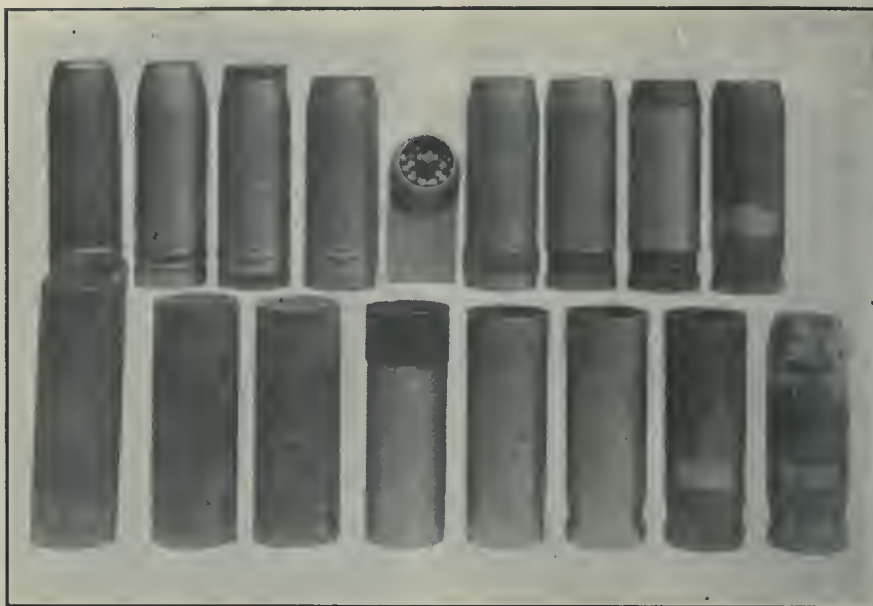
SHRAPNEL SHELLS IN VARIOUS STAGES OF MANUFACTURE AFTER WHICH THEY ARE READY TO BE MADE IN "FIXED AMMUNITION."
