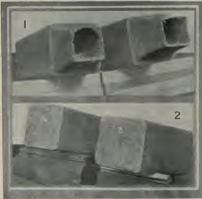
Fig. 1. 18-in. ingots of about 2¾ tons made by the "Hadfield" process. Fig. 2. 18-in. ingots of about 2¾ tons. A—Unsound ingot. B—Piped ingot.
