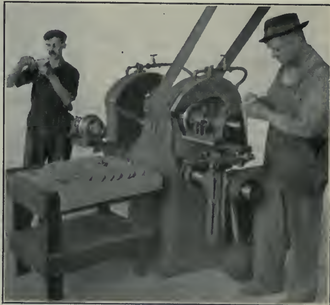
FIG. 2. GRINDER SHOWN EQUIPPED WITH ROTARY CHUCKS AND HOODS.
