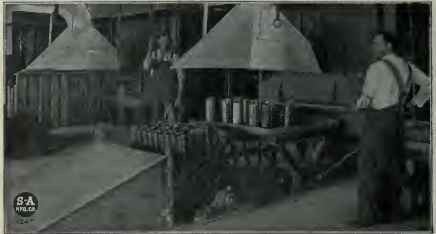
FIG. 1. CARTRIDGE CASES BEING PICKED OFF PAN FROM ANNEALING FURNACE AND LOADED INTO WIRE BASKET ON CONVEYOR.
