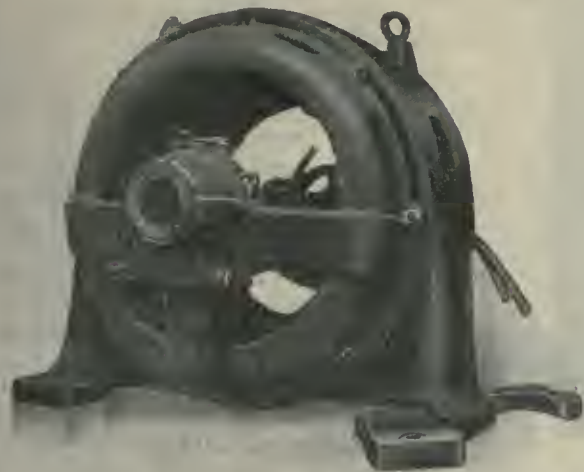
BROKEN FOOT OF ELECTRIC MOTOR.
