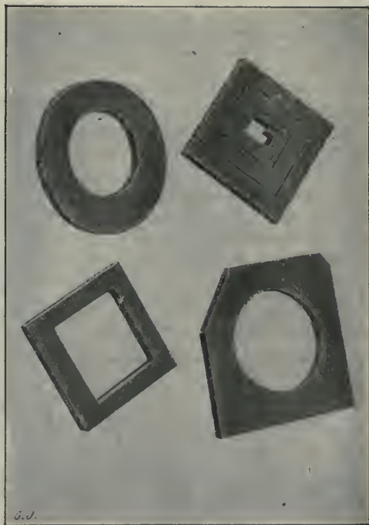
EXAMPLES OF CUTTING DONE WITH OXY-ACETYLENE BLOW PIPE.
