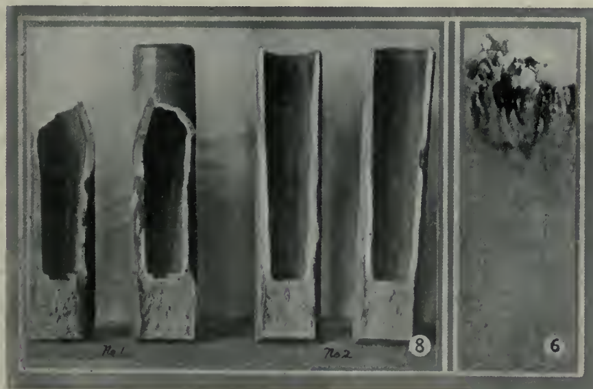
Fig. 6. Etching on axis line to determine amount of segregation. Fig. 8. Shell forgings from blanks (1) and (2) of Fig. 7, split open for inspection.
