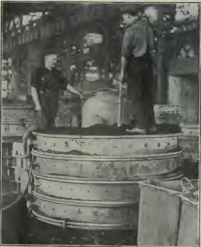
FIG. 11. PREPARING MOLD FOR LARGE STEEL HYDRAULIC CYLINDER.
