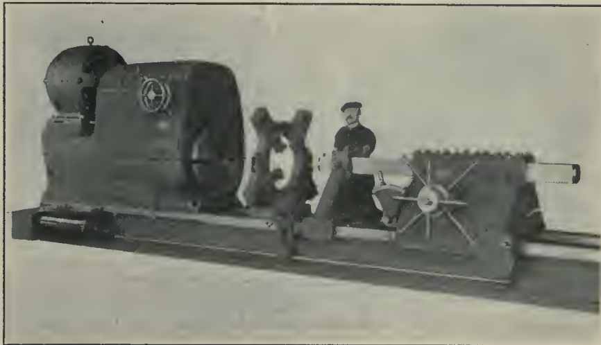
FIG. 15. PROJECTILE BORING LATHE FOR SHELLS FROM 6 IN. TO 12 IN. DIA.
