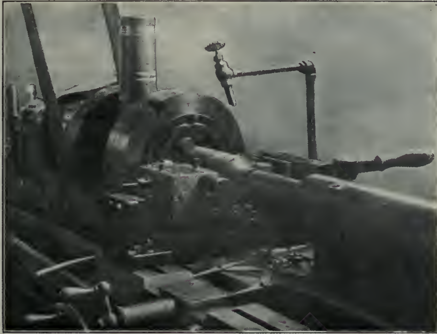
"BERTRAM" WAVING, GROOVING AND UNDERCUTTING ATTACHMENT ON "C.M.C." LATHE.
