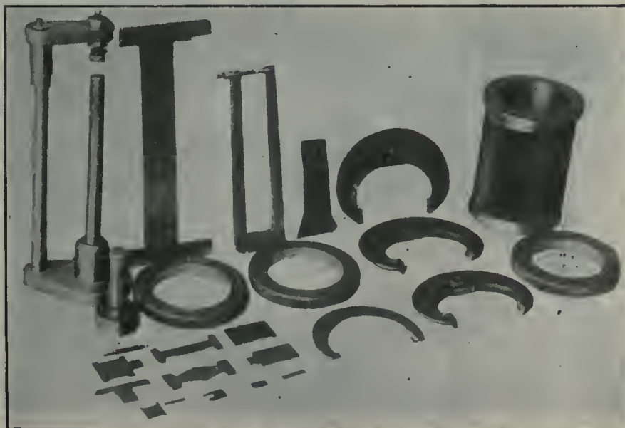
GAUGES USED IN THE MACHINING OF 4.5 HIGH EXPLOSIVE SHELLS.
