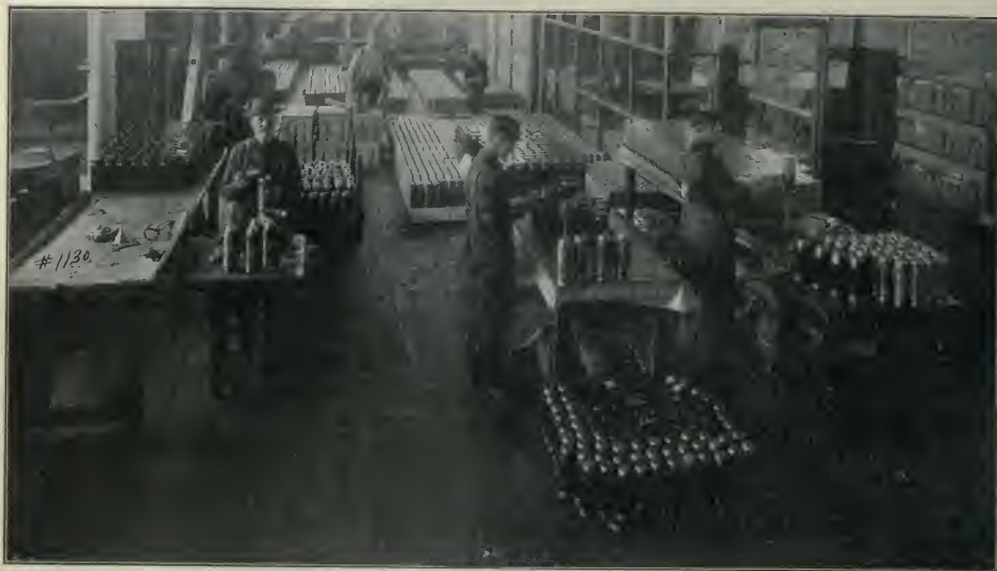
SCENE IN PAINTING DEPARTMENT WHERE SHELLS RECEIVE FINAL TOUCHES BEFORE SHIPPING.
