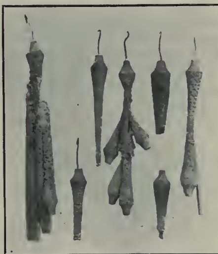
WELDED-UP SCRAP NICKEL ANODES.
