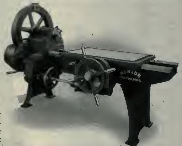
SINGLE SPINDLE MACHINE FOR BORING 6 IN., 8 IN., 10 IN. AND 12 IN. SHELLS.
