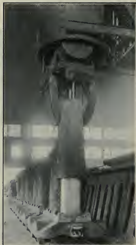
STRIPPING THE MOULD FROM THE HOT INGOT.
