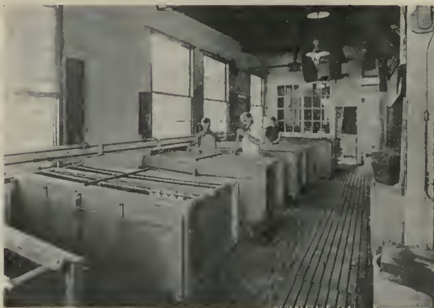
SHOWING ARRANGEMENT OF NICKEL BATHS. POWER SECTION IN BACKGROUND.
