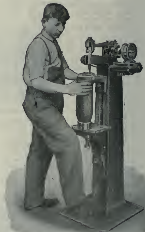
ROTARY VIBRATING RIVETING MACHINE.
