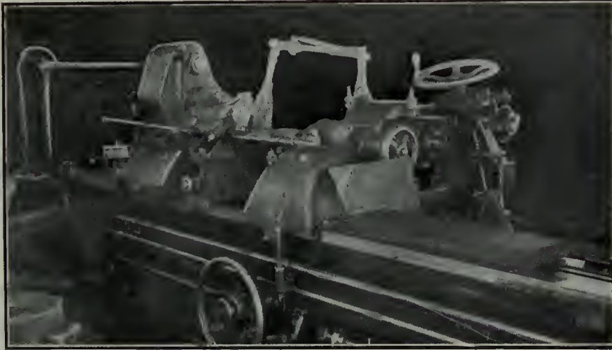
FIG. 9. "LANDIS" GRINDER FITTED UP TO GRIND THE BODY AND NOSE OF THE SHELL AT SAME TIME.
