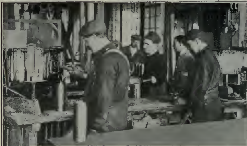
FIG. 11—FILLING SHELLS WITH RESIN; TANKS HEATED BY ELECTRICITY
