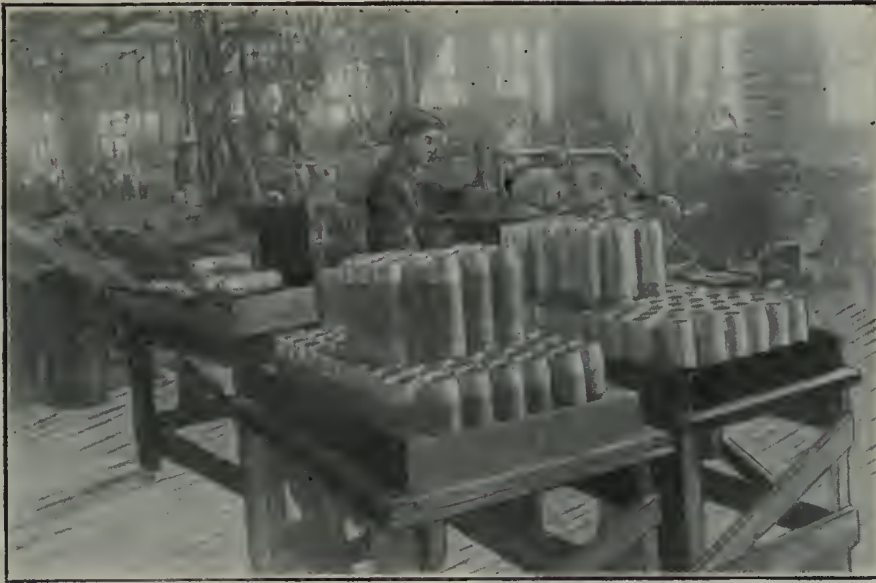
FIG. 21. GRINDING SHELL BODIES AND NOSES.
