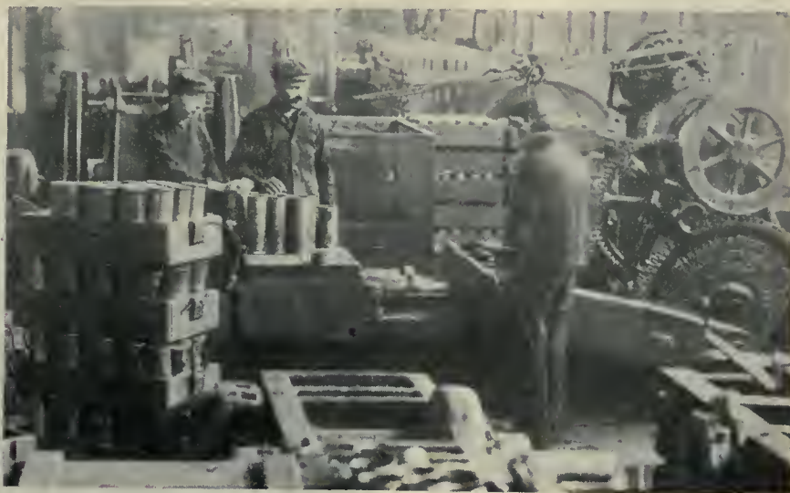
FIG. 11. TAPERING CARTRIDGE CASES ON A BULLDOZER.
