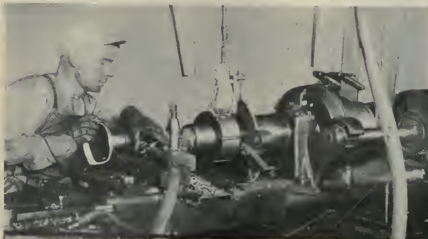
FIG. 15. RIVETING-IN SHELL BASE PLATES.
