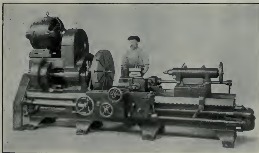
FIG. 4—SHOWING A 30-IN. DOUBLE BACK-GEARED ENGINE LATHE EQUIPPED FOR WAVING AND GROOVING COPPER BAND SEAT OF SHELLS.
