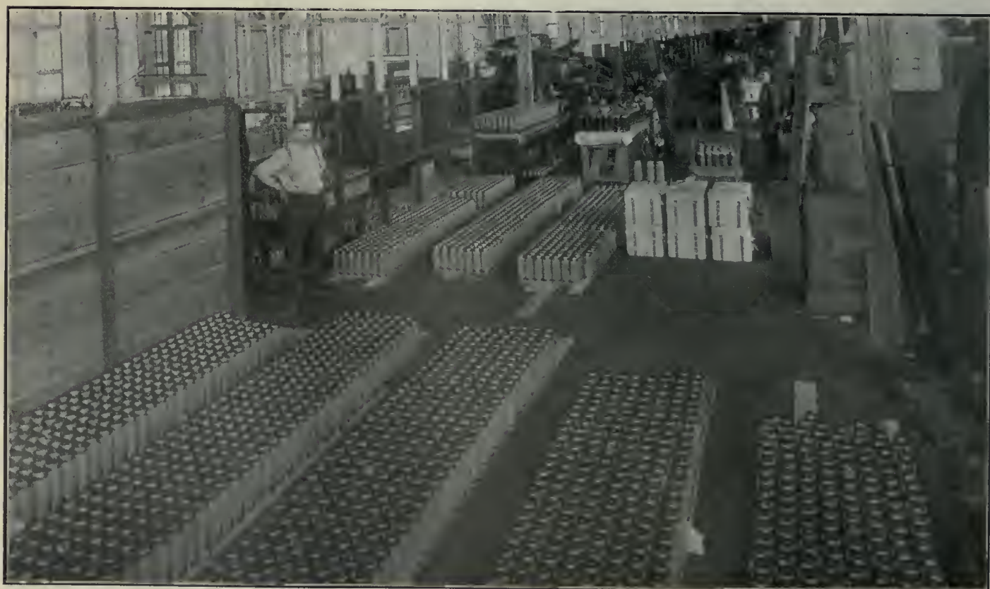
COMPLETED SHELLS, INSPECTED AND PAINTED, READY FOR BOXING AND SHIPPING.
