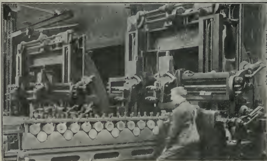
FIG. 13. FACING OFF BASES OF 4.5 HIGH EXPLOSIVE SHELLS.
