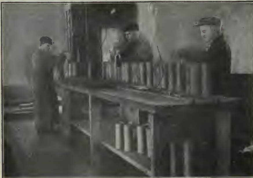
FIG. 14. GOVERNMENT INSPECTORS AT WORK ON 18-PDR. SHRAPNEL FORGINGS.
