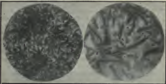
A. CLOSE EVEN GRAIN. FIG. 1. B. OPEN IRREGULAR GRAIN.
