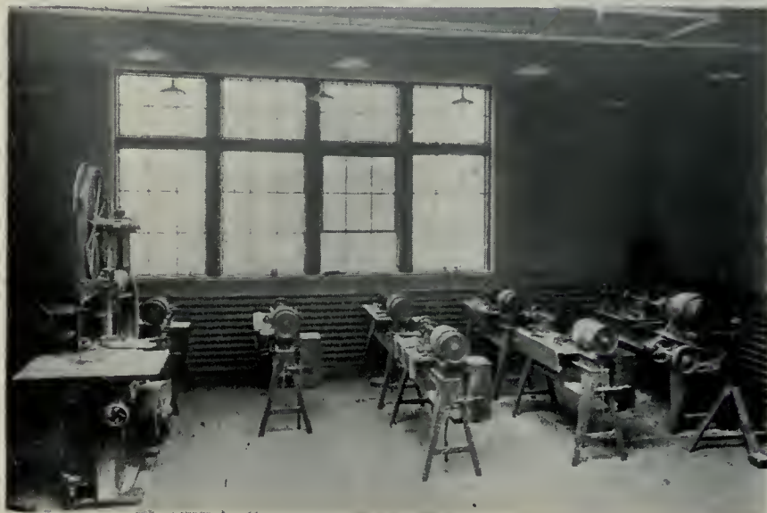
DEPARTMENT OF SHOPWORK. GROUP OF MOTOR HEAD WOODTURNING LATHES IN PATTERNMAKING SHOP.
