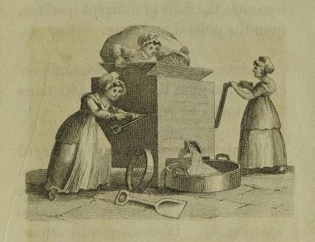
repeatedly scratched with a mill-bill, to renew the necessary roughness for cutting the grain; there are, also, furrows cut from the eye of the stones to the skirts, in order to carry the meal forward as it becomes ground; the meal is then passed through a cylinder covered with wire\* of different fineness, within which, a set of brushes
