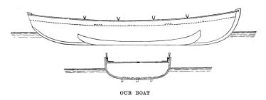
great success; it was strong and elastic enough to resist the pressure of the floes; but for the future I should be inclined to recommend single boarding instead of double, not only because in the former case the boat is easier to repair, but because the intervening space is liable to hold water and increase the weight. Again, I found that the added runners were really of very little use, while they were always liable to get nipped in the ice and thus help to destroy the whole boat.
