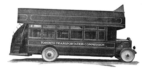
Under the sponsorship of established transportation systems, motor buses were soon designed and equipped to provide safer and more comfortable accommodation for the passengers. Bus number 17, the first pneumatic tired bus purchased by the Toronto system, marks one stage in this development. When it was placed in service in 1924, the passengers who had ridden on solid tired buses thought that number 17 was the last word in bus development.
