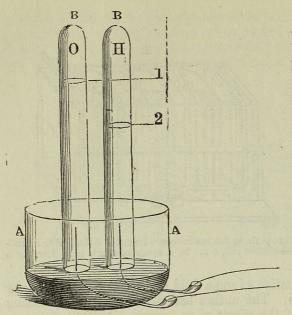
Fig. 138. AA. A finger glass with two holes drilled to pass the wires through, which are imbedded in cement up to the platinum plates. BB. Glass tubes, closed at one end and open at the other, which are placed over the platinum plates to receive the liberated oxygen and hydrogen. The scale at the side shows the respective volumes of two of H to one of O.
