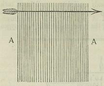
Fig. 410. A A. A number of square tubes placed upright. The arrow shows the direction of the section to obtain a figure like wire gauze. side, but the flame is cut off from the mouth of the jet by the cooling action of the wire gauze. The same experiment reversed, by holding the gauze over the gas burning from the jet, shows still more decidedly that flame will not pass through the metallic tissue. (Fig. 410.)
