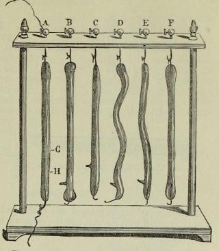
Fig. 248. A, B, C, D, F, F. Various tubes of different kinds of glass, and containing gases and vapours. Each tube has a platinum wire inserted at both ends, with which the contact is made with the coil. The tube A contains mercury, which has been boiled in it, and the air expelled. By moving the conducting wire to G or H, the light which otherwise passes through the whole of the tubes stops at these points.
