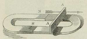
Fig. 203. The horse-shoe magnet, and another one unmagnetized, placed end to end; the one shaded and lettered m and s is the magnet. A A. The piece of soft iron moved in the direction of the arrow.
