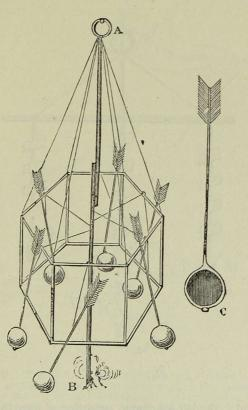
Fig. 115. A. Ring attached to balloon, carrying an hexagonal framework with six shells. B. Hollow fuse, which burns slowly up to the strings, and detaches each shell in succession. c. Section of shell. The shaded portion represents the gunpowder.
