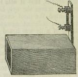
Fig. 241. Microphone mounted on sound-box.
