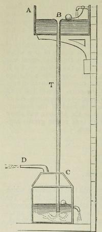
Fig. 81. Model of the apparatus for drawing down air. A, eistern of water, supplied by ball-cock, and kept at one level, so that the water just runs down the sides of the tube, and draws down the air in the centre, B c. The vessel to which the air and water are conveyed by a gutta-percha tube, r. There is another ballcock to permit the waste water to run away when it reaches a certain level; the end of the pipe always dips some inches into this water, whilst the air escapes from the jet, D.
