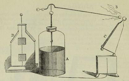
Fig. 182. A. Charged Leyden jar with balanced wire and wool at B, representing a thundercloud. c. The obelisk overturned with the discharge. D. Another model of the gable end of a house; the square pieces of wood fly out when the continuity of the conductor is broken.
