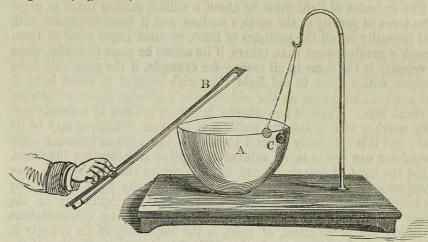
Fig. 279. A. The finger glass. B. The violin bow. C. The ebony ball. The dotted ball shows how it is repelled during the vibration of the glass.
