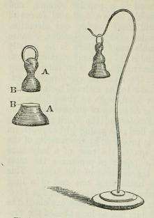
Fig. 75. AA. Two pieces of lead, scraped clean at the surfaces BB. c. Stand, supporting the two pieces of lead attached to each other by cohesion.
