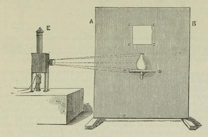
Fig. 303. A B. Portable screen of light framework, covered with black calico. c c c c. Square aperture just above the shelf, D D, upon which the object—viz., a bottle half full of water—is placed. E. Duboscq lantern to illuminate the object at D D.
