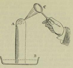
Fig. 98. A. Glass vessel full of mercury, conserved equal scientific glory in his taining the red precipitate at the top, and stand-masterly experiments, through ing in the dish B, also containing mercury. c. The burning-glass concentrating the sun's rays on the which he discovered that the red precipitate, being Priestley's original experi-
