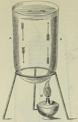
Fig. 416. A A. Inverted glass shade containing water and some paper pulp. B. Burning spirit lamp placed under *one* side of the glass; the pulp shows the rising of the heated water and the sinking of the cold, in the direction indicated by the arrows.
