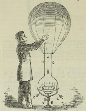
Fig. 402. A B. Wessel's gas stove, with ring of gas jets air balloons. (Fig. 402.) lighted inside; the air rushes in the direction of the arrows, c c, and escaping at the top of the chimney, D D, soon fills the air or fire balloon, which is usually made of paper.
