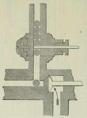
Fig. 418. The charging tube and gun-barrel of steam gun.
