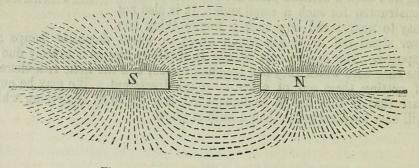
Fig. 270. The curved lines of magnetic force.
