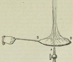
Fig. 433. A. Jet discharging high-pressure steam B B. Lighted torch held round the escaping steam the flames from the former all rush into the latter.
