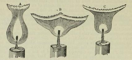
Fig. 273. Effect of magnetism on candle-flame between the poles of the magnet.
