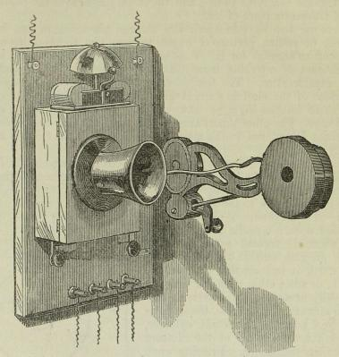
Fig. 237. Exterior view of Edison's loud-speaking telephone.
