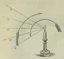
Fig. 288. The rays of light marked A B C D E proceeding from a lighted candle or oxy-hydrogen light. The arrow pointing to the right shows how these rays are crossed in jumping up to the ceiling; and the second arrow, pointing to the left, shows the reverse.
