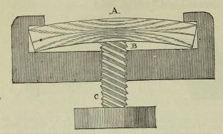
Fig. 387. A B. Bar of glass under the pressure of the screw c, and appearance of bands or fringes of coloured light, which entirely disappear on the removal of the screw. An effect, of course, only visible by polarized light.
