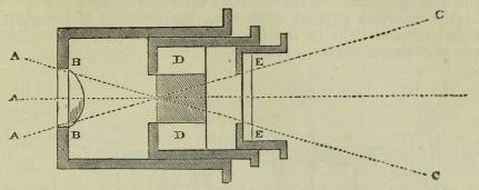
Fig. 389. AAA. Polarized light. B.B. A lens of short focus, transmitting a cone of light with an angle of divergence for its rays, c c, of 45°. D.D. The crystal of topaz, Iceland spar, or nitre. E.E. The slice of blue tourmaline for analysing.
