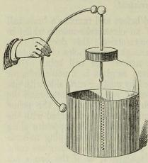
Fig 180. The Leyden jar and brass wire discharger.
