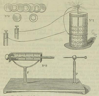
Fig. 252.—No. 1. Spangled Leyden jar. No. 2. Hearder's apparatus for measuring the length of spark for Leyden jar and coil. **PP.** Glass pillars. No. 3. Two best forms of spangles to paste on a Leyden jar.
