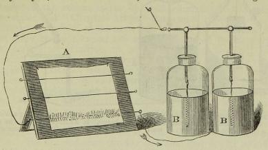
Fig. 181. A. Mahogany board with a sheet of white paper and three pairs of brass wires and balls fixed in the wire, three on each side. The thin wires are stretched between the oalls, and the lower one is in course of deflagration. B. Charged large Leyden battery of two jars; the arrows indicate the path of the electricity.
