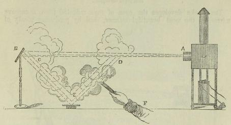
Fig. 305. A. Rays of light slightly divergent issuing from the lantern, and received on a little concave mirror, which brings the rays almost parallel, and reflects them to E, a piece of looking-glass, from which they are again reflected. c is the incident, and p the reflected rays. F. Smoke from brown paper.
