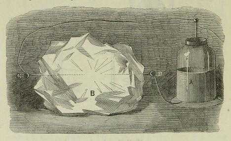
Fig. 256. A. The Leyden jar. B. Large lump of alum, with a hole bored through it in a line with  $c \ D$ . The discharging wires are brought within three-eighths of an inch of each other, and the whole crystal is lighted up with the brilliant electric sparks.
