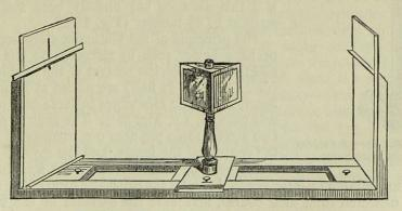
Fig. 357. Wheatstone's reflecting stereoscope.
