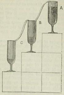
Fig. 82. Geber's filter. A. The solution of acetate of lead. B. The dilute sulphuric acid. c. The clear liquid, separated from the sulphate of lead in B.
