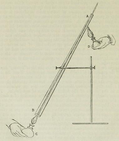
Fig. 420. A B. The glass tube. c. The spirit lamp, with a very large wick; if a little ether is mixed with the spirit in the lamp it increases the length of the flame. D. The effect of the ascension of air, increased by warming the top of the tube with the lamp D.
