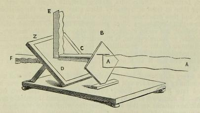
Fig. 384. A.A. Card model of a beam of polarized light coming from the first bundle of plates of glass, shown at Fig. 326, p. 339. B. Model of the film of selenite, which divides or dipolarizes the ray A A into c and D, which, interfering by means of the second bundle of plates of glass called the analyser z, produce reflected chromatic effects by interference at E, and refracted effects at F.
