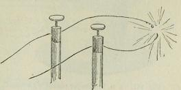
hot that it melts into a Fig. 249. Melting of the iron wire. little globule of liquid iron, and if paper is held between the wires it rapidly takes fire. (Fig. 249.)
