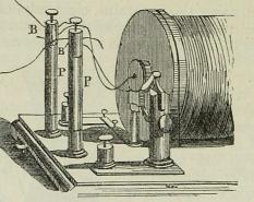
Fig. 247. End of coil where the experiments are performed. B.B. Connecting screws and wires passing to the exhausted globe, c. The screws are supported on insulating glass pillars, P.
