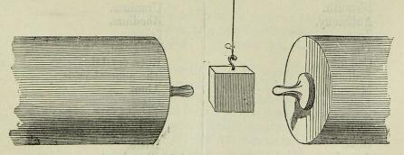
Fig. 271. A cube of copper suspended between the poles of a powerful electro-magnet.
