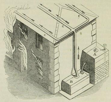
Fig. 156. A. Tank containing acid, communicating by a pipe with  $\mathbf{B}$ , half filled with chalk and water.  $\mathbf{c} \mathbf{c} \mathbf{c} \mathbf{c}$ . Pipes conveying carbonic acid from the generator  $\mathbf{B}$ , to the ceiling, where it is discharged from numerous holes on the fire beneath.
