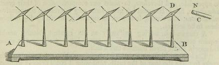
Fig. 281. A B. Series of needles arranged as described. c. The bar magnet, with the north pole N towards the needles. The dotted lines show the direction gradually assumed by all the needles, commencing at D.
