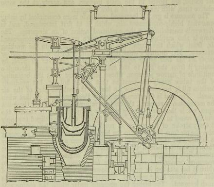
Fig. 403. Stirling's air engine.
