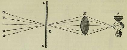
Fig. 360. The stereomonoscope.
