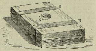
tion of chloride of Fig. 135. A. Circular hole in the upper piece of wood, a similar one being perforated in the lower one. B.B. The strong india-rubber bands. The bleaching solution is poured into A
