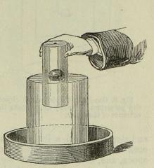
Fig. 7. The orange has entered the glass vessel, and the air having passed from the orifice, no water overflows.
