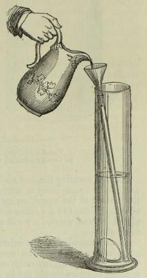
Fig. 66. A vessel half full of water, and as the brine is poured down the tube the egg gradually rises.
