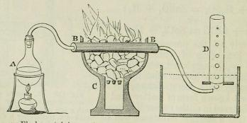
Fig. 111. A. Flask containing water, and producing steam, which passes to the ron tube, B B, containing the iron borings heated red hot in the charcoal stove c. The hydrogen passes to the jar D, standing on the shelf of the pneumatic trough.
