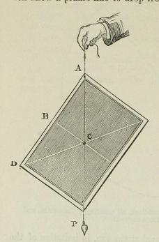
Fig. 42. A B D. The three points of suspension. C, The point of intersection, and, therefore, the centre of gravity. P, The line of plummet.
