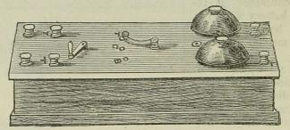
Fig. 233. Telephone bell and shunt.
