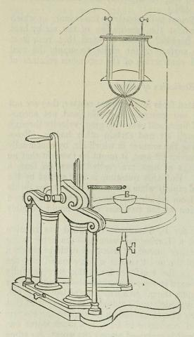
Fig. 425. The air-pump and receiver, containing at  $\blacktriangle$  the electric light in the focus of a concave mirror, and at B a delicate thermometer, also in the focus of a concave mirrov.
