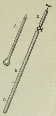
Fig. 80. A. Ordinary glass water hammer. B. Copper tube ditto, showing exhausting syringe at D, the height of the water at B, and the end to be placed in the fire at G and fall. The experiment may be rendered still more instructive by turning the cock and admitting the air, which rushes in with a whizzing sound, and on shaking the tube the metallic ring is no longer heard, but it may be again restored by attaching a small air syringe or hand pump, and removing the air by exhaustion. (Fig. 80.)
