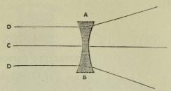
(Fig. 321.) These facts are well shown with the aid of the lantern and electric light. The rays of light Fig. 321. A B. A double concave lens. c Is a ray of light which falls perpendicularly on A B, and passes through without any alteration of its course. D D. Rays falling at an angle on A B, are refracted and diverged
