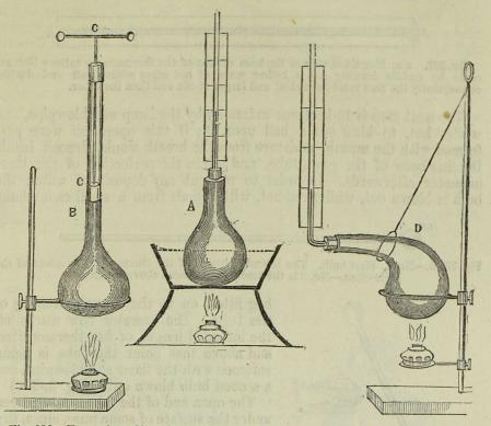
Fig. 396. Expansion of liquids shown at  $\triangle$  by the coloured water rising in the tube from the flask, which is quite full of liquid, and heated by boiling water. B. The expansion of the water heated by the spirit-lamp is shown by the rising of the piston and rod c c. D represents a retort filled up like  $\triangle$  to show the expansion of a liquid by heat.
