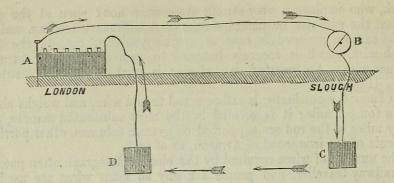
Fig. 216. A. The battery. B. The instrument. c. Earth plate at Slough. D. Earth plate at London. The arrows show the direction of the electric current.
