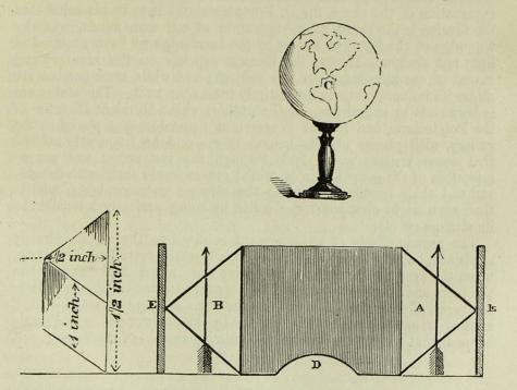
Fig. 362. Horizontal section of the pseudoscope, showing at  $\blacktriangle$  B two prisms placed against a block of wood about two inches long and one inch and a half wide, and cut out in the centre to admit the nose at D. The eyes are supposed to be looking at the globe, c, in the direction of the arrows. E B. Brass plates blackened, which shut out the side light, and assist in keeping the prisms in position.
