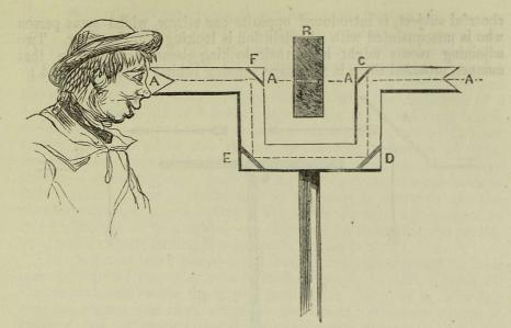
Fig. 292. A A A A. The apertures through which the spectator first looks. B. The piece of wood, four inches thick. C, D, E, F, are four pieces of looking-glass, so placed that rays of light entering at one end of the tube are reflected round to the other where the eye of the observer is placed.
