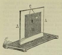
Fig. 179. AA. Glassplate or stand coated with tintoil on each side, B. C. Wire with pith balls oscillating during the discharge of the glass plate.
