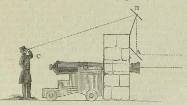
Fig. 293. A picture of enemy's battery is supposed to be on the mirror, A, whence it is reflected to B, and from that to the artilleryman at c.
