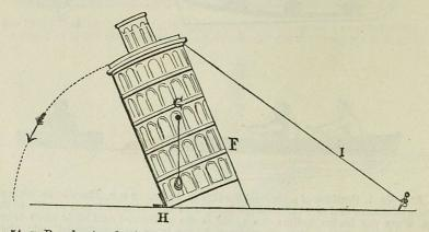
Fig. 54. F. Board cut and painted to represent the leaning-tower of Pisa. G. The centre of gravity and plummet-line suspended from it. H. The hinge which attaches it to the base board. I. The string, sufficiently long to unwind and allow the plummet to hang outside the base, so that, when cut, the model falls in the direction of the arrow.
