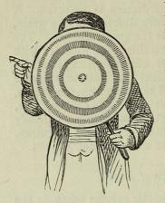
Fig. 353. Design for the phenakistiscope. The spectator is supposed to be looking towards a mirror through the slits. It is supported by a handle through the centre, round which it is twirled by the other hand.
