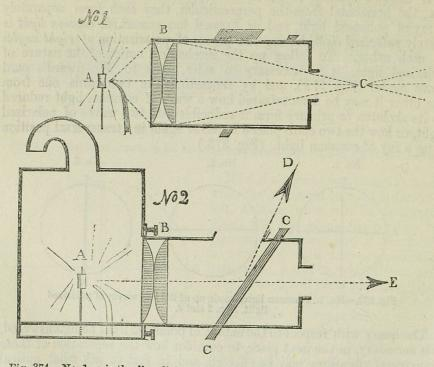
Fig. 374.—No. 1. A is the lime light. B. The condenser lenses. c. The beam of common light. Here the glass plates are removed.—No. 2. A. Lime light. B. The condenser lenses. c. The bundle of plates of glass at an angle of  $56^{\circ}45^{\circ}$ . D is the ray of light polarized by reflection from the glass plates, c c, and E is the beam of polarized light by single refraction, having passed through the bundle of plates of glass, c c.
