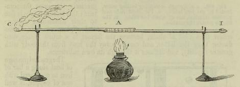
Fig. 405. c. Copper wire bound at  $\mathbf{A}$  to  $\mathbf{I}$ , an iron wire. After the heat of the lamp has been applied for about five minutes the heat travels to c first, and ignites the bit of phosphorus placed there. After some time has elapsed the phosphorus at  $\mathbf{I}$  also ignites.
