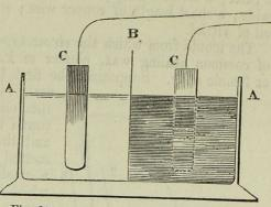
Fig. 190. AA. A glass trough containing the salt dissolved in water, and divided temporarily with a bit of cardboard, B. c c are the two platinum plates connected with the battery, and the shaded side is supposed to represent the liberation of the iodine.
