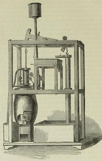
Fig. 412. Model of the Newcomen engine, in which the furnace and boiler, the steam cylinder, beam, water-pump, and elevated cistern of water, are apparent.
