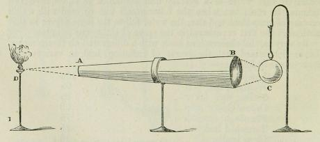
Fig. 429. A B. The cone of paper, gilt inside. c. The red-hot ball. D. Stand with wood supporting a slice of phosphorus, which is brought into the focus of the rays of heat reflected through the cone.
