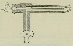
Fig. 122. Daniell's jet. o o. The stop-cock and pipe conveying oxygen, and fitting inside the larger tube  $\mathbf{H}$  **H**, to which is attached a stop-cock, **H**, connected with the hydrogen receiver. A. The orifice near which the gases mix, and where they are burnt.
