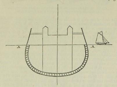
Fig. 78. Transverse section of *Great Eastern*, showing the cellular construction from keel to water-line,  $\triangle A$ .
