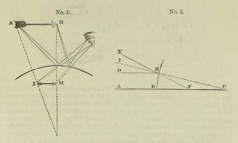
Fig. 296. A B, D H. (No. 2) represent two parallel rays incident on the convex surface B H, the one (A B) perpendicularly, the other (D H) obliquely. c is the centre of convexity. H E is the reflected ray of the oblique incident one, D H; whilst C H I is the perpendicular.
