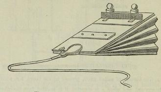
Fig. 123. Gas bag and pressure boards.
