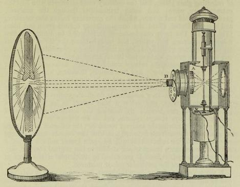
Fig. 383. The electric lamp and lantern of Duboscq, showing the projection of the carbon poles on the disc. This experiment is performed with the help of the plano-convex lens, A, and the rays pass through a very narrow aperture at B.
