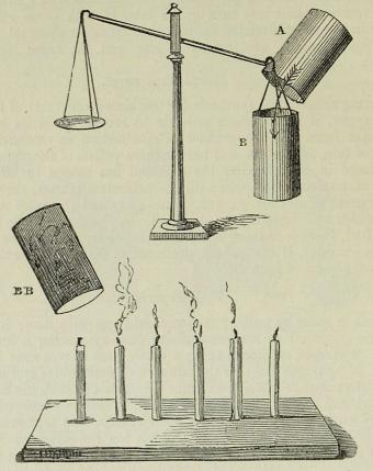
Fig. 152. A. Carbonic acid gas poured out of the tin box into B, the muff-box. B B. Detached muff-box, and candles extinguished by the carbonic acid gas poured from it.
