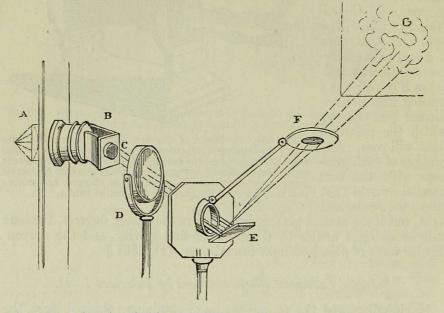
Fig. 382. Duboscq's polarizing apparatus. A. The light and the condenser lens. B. The plates of glass at the proper angle. C. The selenite object. D. The focusing lens. E. The second bundle of plates of glass called the analyser. F. A stop for extraneous rays of light. G. The image of the film of selenite most beautifully coloured.
