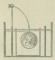
Fig. 194. The gallipot containing the solution of sal ammoniac, with the circular amalgamated zine with wire and binding screw to which the medal is attached, and contained in the porous vessel holding the silvering solution and medal.
