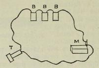
Fig. 244. The microphone in circuit with a battery and telephone.
