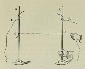
Fig. 195. A A. Two ring stands with the battery wires B B (which should be a convenient length) attached. c. Platinum wire, fixed end. D. The other end held in one hand and shortened as the stand is moved by the other hand.
