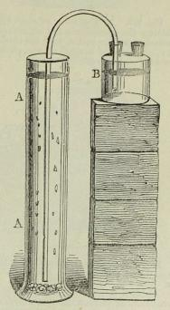
Fig. 15°. A A. Tall glass nearly full of water; at the bottom are the ehlorate of potash and phosphorus. B. Wolfe's bottle and syphon, conveying the oil of vitriol to bottom of A A.
