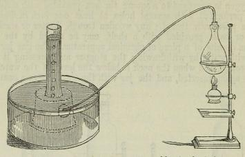
Fig. 95. Preparation of oxygen from  $\begin{cases} chlorate of potash, \\ oxide of manganese. \end{cases}$
