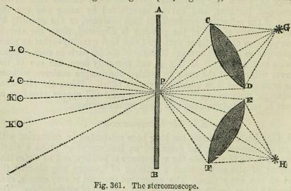
lenses (C D, and E F) arranged in such a manner that they will project images of the stereoscopic pictures, G H, at the same point on the screen, A B.
