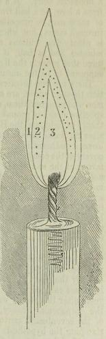
Fig. 278. A candle flame. 1. Outer flame. 2. Inner flame. which is badly supplied with oxygen, and where the carbon is deposited and *ignited*. 3. The interior, containing unburnt gas. consists of a cylinder of wood one inch in diameter and seven inches long, placed in the angle of a black box with the electric lamp inside, so that three-fourths of the cylinder are visible outside, and the remaining fourth exposed to the interior electric light.
