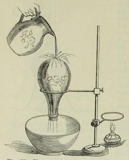
Fig. 437. The paradoxical experiment of water boiling by the application of *cold* water.
