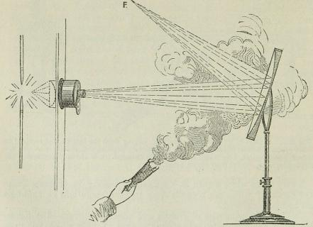
Fig. 307. The smoke shows rays of light falling on the concave mirror. In this experiment attention should be directed to the bright point, E, the focus where the convergent rays meet.
