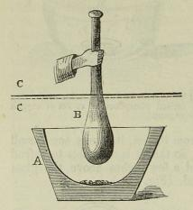
Fig. 160. A. The iron mortar containing the phosphorus and chlorate of potash. B. The pestle, with the shield, o c, composed of a circle of wire gauze, covered with one of cardboard.
