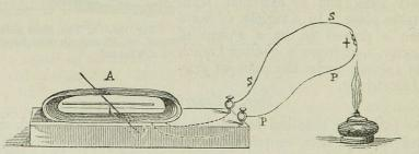
Fig. 167. A. The galvanometer needle, with wires attached. s, s. Silver wire joined to P, P, the platinum wire. The heat of the spirit-lamp is applied at the point of juncture, +.
