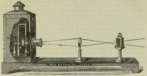
Fig. 349. Apparatus for showing spectrum on screen.
