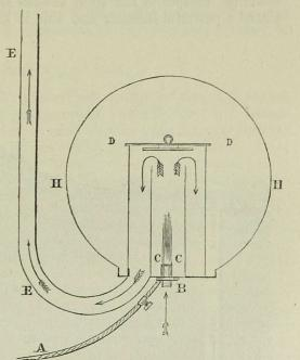
Fig. 423. A B. Gas pipe and argand burner; the air enters, as usual, up the centre of the argand. c c. The first glass chimney open at the top. D D. The second glass chimney closed at the top, with a disc of double talc, and fitting over c c, and leaving a space between the two glasses, down which the air passes, and into the ventilating tube, B E. H H. The ground-glass globe closed at the top, and surrounding the whole.\*
