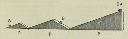
Fig. 41. P P. Inclined planes, gradually decreasing in height, cut out of inch mahogany, with a groove at the top to carry an ordinary marble. B B B. Different positions of the marble, which starts from B A. D
