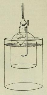
Fig. 9. Gas-jar; stop-cock open; the air passes, the water enters, and the potassium is inflamed.
