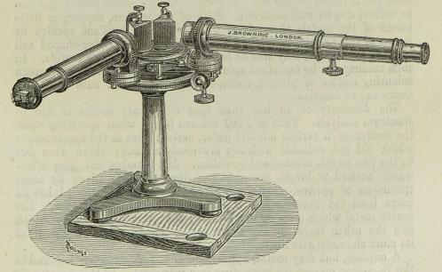
Fig. 351. Spectroscope with two prisms.
