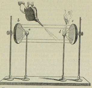
Fig. 404. Heat reflected by mirror, but not blown away by air from bellows.
