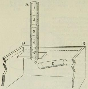
Fig. 109. A. Gas jar divided into five equal parts. B B. Section of pneumatic trough, to show the decantation of gas from one vessel to another. The gas is being passed from c to A, through the water.
