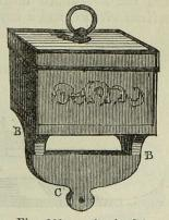
Fig. 201. A loadstone mounted in brass or silver, with the iron cheeks BB attached. c. The bit of soft
