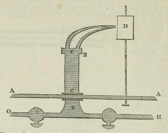
Fig. 124. AA. Board to which в в is fixed. o. Oxygen pipe. н. Hydrogen pipe. сс. Space filled with wire gauze. D. Lime cylinder.
