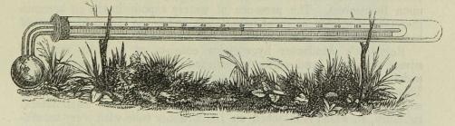
Fig. 426. Negretti and Zambra's terrestrial radiation thermometer. The bulb of this instrument is transparent, and the divisions engraved on its glass stem. In use it is placed with its bulb fully exposed to the sky, resting on grass, with its stem supported by little forks of wood, and protected from the wind.
