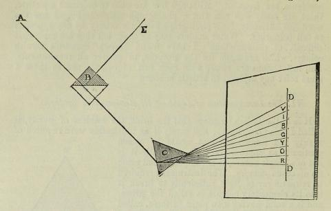
Fig. 348. A. The ray of light passing through two prisms B placed base to base. In this position the light passes through to the second prism, c, without alteration. At  $\sigma$  the decomposition of light occurs, and the spectrum is shown at D D. The top prism at B used singly would reflect the ray to B without decomposing it into the coloured rays.
