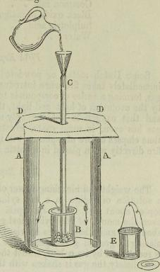
enough chlorine has been generated, or some very finely-pow- The small one, containing the chloride of lime. dered antimony will demonstrate c. The tube and funnel down which the dilute the same result. Thus, with a over top of large glass, with hole in centre to few beaker glasses, some chlo- admit the tube. E. The little beaker used as a ride of lime, sulphuric acid, a
