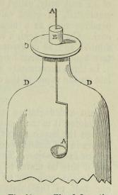
Fig. 99. A. The deflagrating spoon. B. The cork. C. The zinc, or brass, or tin plate. DD.
