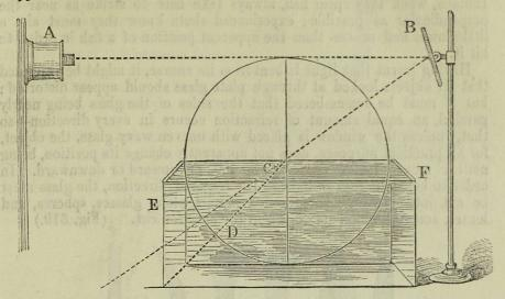
Fig. 317. A. Duboseq lantern. B. The mirror. B c. The incident ray. C D. The refracted ray. E F. Tank, containing water up to the horizontal line of the circle.
