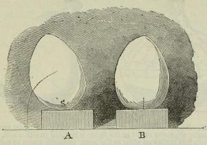
Fig. 45. A Represents the egg in its natural state, and, therefore, in unstable equilibrium; n, another egg, with the surface, s, flattened, by which the centre of gravity is lowered, and if not disturbed beyond the extent of the point of support the equilibrium is stable.
