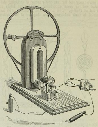
Fig. 261. Clarke's magneto-electrical machine.
