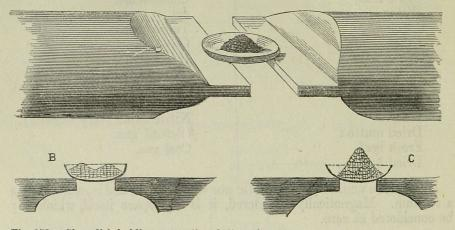
Fig. 272. Glass dish holding magnetic solution of iron, and placed in the magnetic field.
