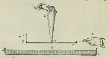
Fig. 178. A A. Large circular tin or brass disc with turned-up edge half an inch deep, and containing the resinous mixture B, which is rubbed with the warm flannel. c c. The upper plate supported by the glass handle D, a pith ball attached to a wire shows the electrical excitation, and the spark is supposed to be passing to the hand E.
