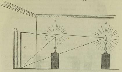
Fig. 284. A. The lamp. B. The candle. c. The rod throwing the two shadows, marked D and B, on a white wall or a sheet of paper.
