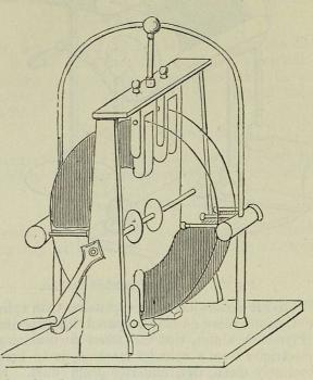
Fig. 173. Woodward's double plate electrical machine, giving a much larger quantity of electricity than Fig. 167.
