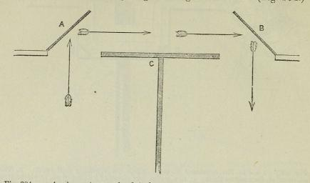
Fig. 294. A. A mirror at an angle of 45 degrees. The arrows show the direction of the reflected image. B. The second mirror, also at an angle of 45 degrees; the face of the person looking in at  $\underline{A}$  is reflected at B. c is the partition between the rooms.
