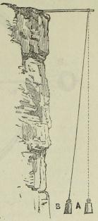
Fig. 12. The Schichallion Rocks. The dotted line and weight  $\land$  represent the ordinary position of a plumbline, whilst the line of the weight  $\bowtie$  indicates (of course, with some exaggeration) the attractive power of the mass of the rock drawing it from the perpendicular. called "the industrious fleas," and our jumping would be something marvellous.
