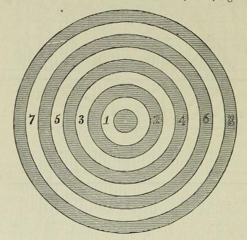
Fig.366. Appearance of Newton's rings when produced in yellow light, 1, 3, 5, 7, being the yellow rings, and 2, 4, 6, 8, the dark rings. Light by the odd numbers; darkness by the even numbers. The central spot, where the two surfaces are in contact, is dark.
