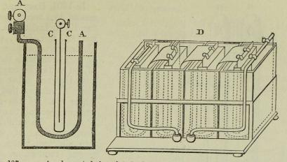
Fig. 187. A A. Amalgamated zinc plate in flat earthenware trough. Attached to a binding screw 15 the platinum plate in porous cell, c c. D. A series of single cells forming a Grove's battery.
