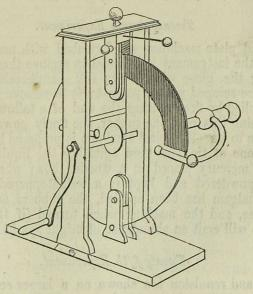
Fig. 172. The ordinary plate electrical machine. O 2 trical purposes, in consequence of the decomposition of the surface from imperfect manufacture and the liberation of the alkali. (Figs. 172, 173.)
