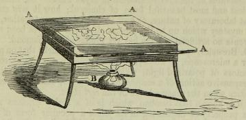
Fig. 149. A A A. The glass plate, with the waxed side downwards, placed on the leaden tray containing the fluorspar and sulphuric acid. B. Spirit lamp.
