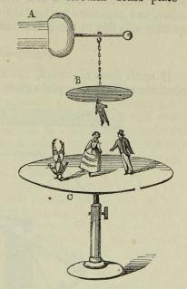
Fig. 175. A. Prime conductor. B. Upper brass-plate. c. Lower ditto. The figures are seen between B and C.
