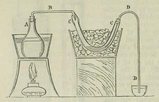
Fig. 161. A. The flask containing the phosphide of calcium and water, and placed in a water-bath heated to  $140^{\circ}$  Fah. B. Bent tube conveying the gas to c c, the U-shaped tube, to which it is attached by india-rubber tubing. c c. The Ushaped tube, surrounded with a freezing mixture. D D. Bent tube, passing into a cup of water to prevent contact with air.
