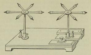
Fig. 197. De la Rue discharger, containing a series of six pairs of different substances, such as charcoal, Fizeau and Foucault iron, lead, zinc, copper, antimony, in six pair of crayon holders, and turning on a centre, so as to be charged at pleasure.
