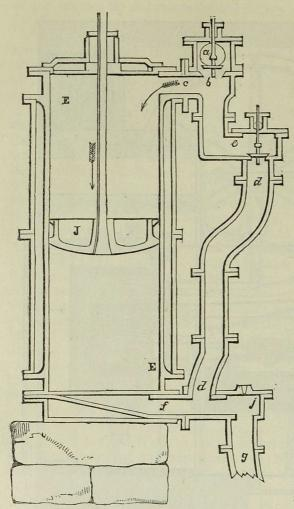
Fig. 444. "BE is the cylinder. J. The piston. a. The steam-pipe. b. The regulating or throttle valve. e. The eduction and equilibrium single valve, performing the functions of both. c. The upper, and f the under, portholes, by which passages only the steam can enter and pass away. d, j, g. The eduction-pipe by which the steam passes from above the piston during every returning stroke to the condenser, a perpetual exhaustion being maintained beneath it."—From BOURNE on the Steam-engine.
