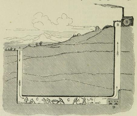
Fig. 424. Section showing the two air-shafts. A. The downcast. B. The upcast. c. One of the working galleries in connexion with the upcast and downcast. D. The furnace at the bottom of the *upcast*. In this sketch one gallery only has been shown, to prevent confusion and to show the principle.
