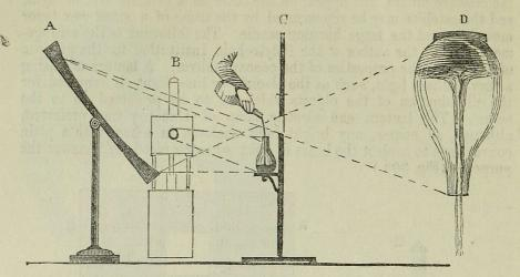
Fig. 304. A. The concave mirror. B. The lantern. c. The portable screen, shelf, and object. D. The inverted image of the bottle filling with water, with the neck downwards, and when thrown on the disc at D producing a most curious illusion.
