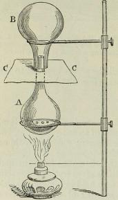
Fig. 136. A. Flask containing iodine heated by spirit lamp. B. Cold flask above to receive the vapour. c c. Sheet of cardboard lamp.
