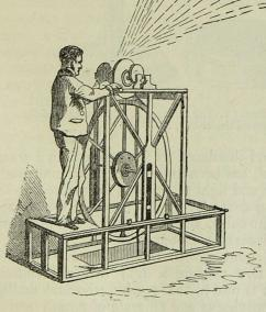
under the action, viz., the friction of a soft iron disc revolving with great velocity against a file or other convenient piece of hardened steel. (Fig. 276)
