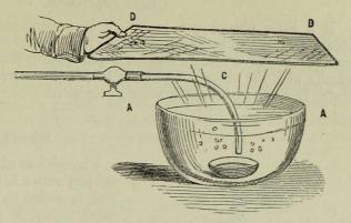
Fig. 158. A A. Finger-glass of boiling water containing a metallic cup with melted phosphorus. c. Jet of oxygen gas. D D. Sheet of wire gauze.
