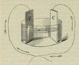
Fig. 184. A single voltaic circle, consisting of a zine and copper plate (marked z and c) in dilute acid. The arrows show the direction of the current.
