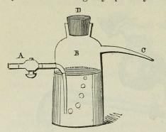
Fig. 120. Gurney's jet. A. Pipe with stop-cock leading from the gas-holder. B. The little reservoir of water through which the mixed gases bubble. c. The jet where the gases burn. D. Cork, which is blown out if the flame recedes in the pipe, c.
