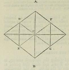
Fig. 380 represents a crystal, the axis of which is the direction  $\_$  B. The dotted lines show the division of the large crystal into four other and smaller ones, each of which has its axis,  $\_$  C, C, B, D, E, F, G; and every line within the large crystal parallel to  $\_$  B is an axis, consequently the term is employed usually in the plural number axes.
