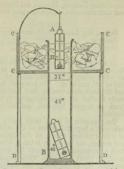
Fig. 400. A B. Long cylindrical glass containing water and two thermometers; the one at the bottom shows a temperature of 40°; the other at the bottom box surrounding the top of the glass. (Fig. 400.)
