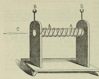
Fig. 199. A A. A glass tube supported on two uprights of wood, with coil of copper wire passing round it, terminating in the balls **B** B. C. Needle to place inside glass tube.
