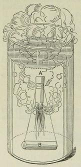
Fig. 101. A. Case of red fire burning downwards, and attached by a copper wire to a bit of leaden pipe B, to sink it. c c. Jar containing water.
