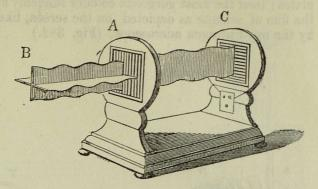
Fig. 381. A. Model of the first slice of tourmaline into which the transversal vibrations, B, are passing; the horizontal wave is absorbed, and the perpendicular polarized one proceeds to the second slice of tourmaline, c, where the bars (the axes) being at right angles to those of A, it is stopped, and cannot pass through until the bars of c are parallel with A.
