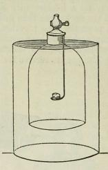
Fig. 8. Gas-jar with stop-stock closed, and potassium in ladle; air prevents the entrance of the water.
