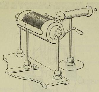
Fig. 171. A cylinder electrical machine.
