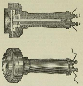
Fig. 231. Prof. Bell's telephone, in elevation and section.
