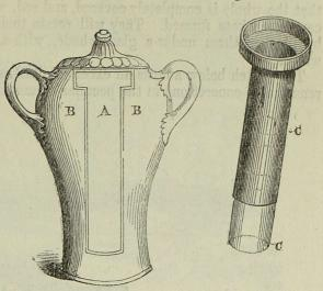
thaws the surrounding Fig. 90. A. The inner cylinder which contains the freezing mixture. B B. The outer one containing spring water. c c. The ice slipping away from the inner cylinder.
