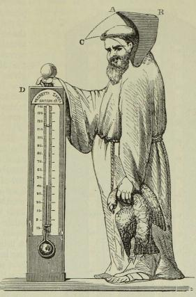
Fig. 427. The monk hygroscope, in which the hood, A B, covers the head to dotted line c in wet weather, and takes various intermediate positions, being quite back and on the shoulders in dry states of the air. A thermometer, D, is usually attached.
