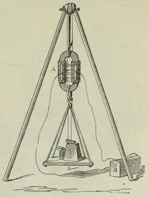
Fig. 204. A. Powerful electro-magnet supporting a great weight. B. The battery.
