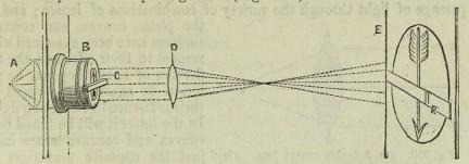
Fig. 318. A. Rays of light from the electric light. B. The cap, with figure of arrow cut out. c. The bar of plate glass. D. The double convex glass to focus E, the image on the disc, and portion refracted at B.
