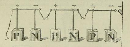
Fig. 177. The lengths of brass wire supported on glass rod pillars indented by blowpipe, so as to retain the brass wires with the pith balls hanging from each series, the letters P and N mean Positive and Negative, and the signs for these terms are placed above. The letters P and N are painted on the blocks which support the glass rods.
