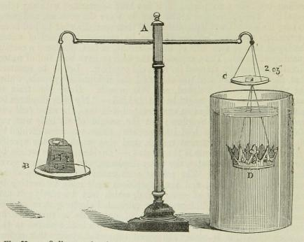
Fig. 68. A. Ordinary pair of scales. B. Scale-pan, containing  $17\frac{1}{2}$  ounces, being the weight of the crown in air. c. Pan, with hook and crown attached, which is sunk in the water contained in the vessel D; this pan contains the two ounces, which must be placed there to make the crown sink and exactly balance B.
