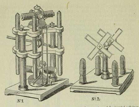
Fig. 212.—No. 1 consists of vertical permanent steel magnets and horizontal soft-iron electro-magnets which rotate.
