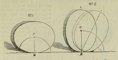
Fig. 44. The point of support. c, The centre of gravity.
