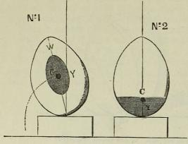
vity. A good billiard-player Fig. 46.—No. 1. Section of egg. c. Centre of gravity. should, therefore, always try x. The yolk. w. The white. No. 2. c. Centre of gravity, much lowered. x. The ball before he engages yolk at the bottom of the egg. to play for any large sum.
