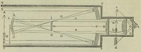
Fig. 309. The Gregorian reflecting telescope.
