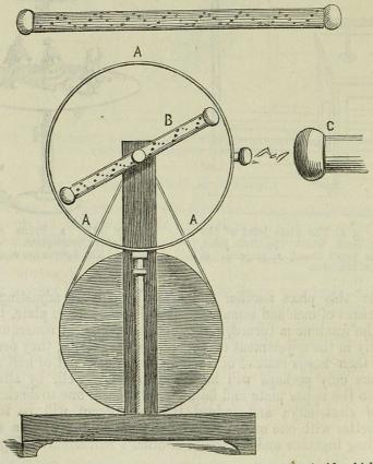
Fig. 176. AAA. A ring of brass wire supported on a glass pillar inside which the spiral tube, B, revolves, and produces beautiful and ever-changing circles of light, when connected with the conductor, c, of the electrical machine.
