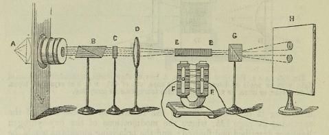
Fig. 390. A. The light and condenser lens. B. Single-image Nicol prism. c. Rock crystal of two rotations. D. A double-convex lens. E E. Faraday's heavy glass. F F. The powerful electro-magnet connected with battery. G. Double-refracting prisms. H. Image, or screen where the deviation of the plane of polarization by the magnetic force is shown.
