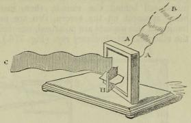
Fig. 375. AA. Model in wood of a bundle of plates comes more apparent. of glass at an angle of 56° 45′. B. Beam of common The same truth is well light, with transversal vibration. c. Light polarized by reflection. D. Light polarized by refraction.
