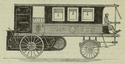
Fig. 430. Hancock's steam omnibus, which ran on the common roads.
