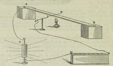
Fig. 395. A B. Compound bar resting on two blocks of wood. The end A is connected with one of the wires from the battery. The circuit is completed and the platinum lamp p ignited directly the bar curves *upwards* by the heat of the spirit lamp, and touches the wire c c connected with the opposite pole of the battery.
