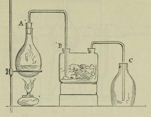
Fig. 130. A. Flask containing the fuming hydrochloric acid, which is gently boiled by the heat of the spirit lamp. B. Tube passing to the Wolfe's bottle, containing pumicestone or asbestos moistened with sulphuric acid. c. Second tube passing into a dry empty bottle, which receives the hydrochloric acid gas.
