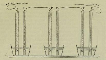
Fig. 126. Grove's gas battery consists of tubes containing oxygen and hydrogen alternately, and having a thin piece of platinum foil, P, inserted by the blowpipe in each glass tube. The foil hangs down the full length of the interior of the glass. Each pair of tubes is contained in a little glass tumbler containing some dilute sulphuric acid, and the hydrogen tube, H, of one pair, is connected with the oxygen tube, O, of the next. w w. The terminal wires of the series.
