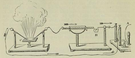
Fig. 253. A. The coil. B. Hearder's discharger, with thin platinum wire, P, hanging between the points. c. Another discharger, and powder going off between the points from the little table. The pillars of the dischargers are glass. The arrows show the direction of the current of electricity.
