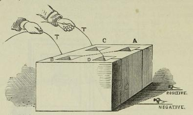
Fig. 225. Block of wood with four holes; the positive terminal is connected with the holes A and B, the negative with c and D; the hollows are filled with mercury. TT are the wires from the telegraph box, and it is obvious that by dipping them alternately into CB and A i) the current is reversed, and the needle deflected right or left at pleasure.
