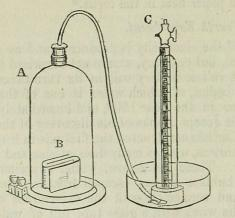
Fig. 189. A. Gas jar with cap and bent tube passing to the graduated tube c; the jar is cemented in the same stand which carries the connecting cups, wires, and platinum plates, which are bent round each other to improve the action of the voltameter.
