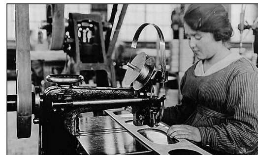
Women sewing wing reinforcement strips at Canadian Aeroplanes Ltd., 1918.
