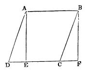
2. What is the content of a field in the form of a rhombus, whose length is 7.6 chains, and perpendicular height 5.7 chains? Ans. 43.32 chains.
