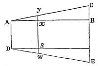
Here A  $x = \frac{1}{2 \text{ B C}} (\checkmark \{ (B \times AD)^2 + 4 \text{ B C} \times AB \times AD = \frac{1}{3} (\checkmark \{ (20 \times 3)^2 + 6 \times 20 \times 60 \} -20 \times 3 = 14 \cdot 64, \text{ the length required.} \}$
