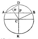
2. If the chord AD of half the arc ADB be 20 feet, and the chord A B of the whole arc 38; what is the length of the arc?  $20 \times 8 - 38 = 122$ ; then  $122 \div 3 = 46\frac{2}{3}$  feet. Ans.
