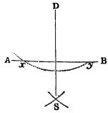
When the point is nearly opposite the end of the given line, and when the given line cannot be conveniently produced.
