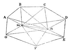
Let m and n be two stations, from which all the marks A, B, C, &c., can be seen, plant the instrument at m and by it, measure the angles A m n, B m n, C m n, &c. Next measure m n, and planting the instrument at n, measure the angles A n m, B n m, C n m, &c. These observations being planned the lines joining the points of external intersection, will give a true map of the ground. The method of finding the content will be shown further on.
