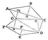
into trapeziums and triangles; measure them separately, as in the two last problems: and the sum of all the separate results will give the area of the whole field.
