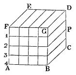
Here,  $4 \times 4 = 16$ , the number of cubes of 1 inch deep is the square E F G D, and as the entire solid consists of four such dimensions, its content is  $16 \times 4 = 64$  cubic inches.
