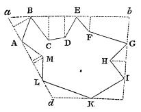
When there are obstructions within the figure, such as wood, water, hills, &c., measure the lengths and positions of the four-sided figure  $a \ b \ c \ d$ , taking care to measure the offsets from the different corners as you go along.
