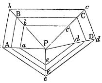
ure  $a \ b \ c \ d \ e$  be similar to the original one, and upon the cequired scale. Or measure all the sides and diagonals of the figure by a scale, and lay down the same measures respectively from another scale, in the required proportion.
