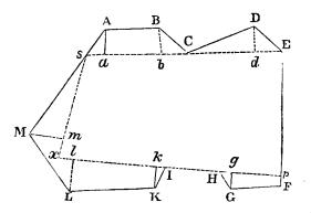
$s \in B$  A, C D E, &c. must be added to the area of the quadralateral  $s \propto F$  E. But when the principal lines are taken outside the figure, the portions included between them and the boundaries of the field are to be deducted from the content of the quadralateral, and the remainder will give the true content of the field.
