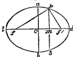
Thus Fig. 15 *atbd* is an ellipse because  $pt + pt'$  is constant; *f* and *f'* are the foci, *c* the centre, *td* the transverse and *ab* the conjugate diameter or axis, *sm* is an ordinate and *sp* a double ordinate, *tm* and *md* are the abscisses to the ordinate *sm*.
