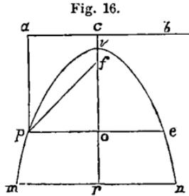
Thus if the curve  $mn$  is such that any point  $p$  in it is equally distant from the point  $f$ , and the line  $ab$ , that is, if  $pa$  is equal to  $pf$ , then the curve  $mn$  is a parabola. Also  $f$  is the *focus*;  $po$  is the *ordinate*, and  $pe$  the *double ordinate* or *base*,  $v$ , is the *vertex*, and  $ov$  is the *absciss*. The double ordinate through  $f$  is called the *parameter*.
