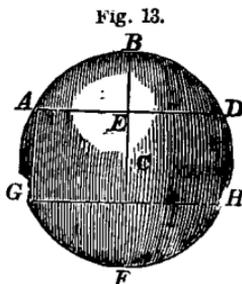
51. A *segment* of a sphere is a part of it cut off by a plane; a segment of a pyramid, cone, cylinder or other solid, with a plane base is a portion cut off from the top by a plane parallel to the base.
