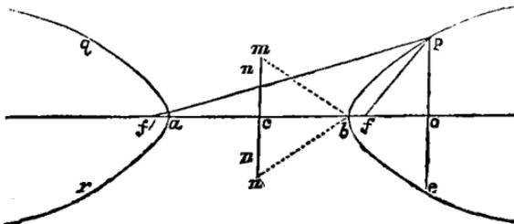
Thus if any point  $p$  in the curve  $pbe$  is such that  $pf' - pf = ab$ , a given line, then the curve  $pbe$  is an hyperbola. Also  $f$  and  $f'$  are the *foci*,  $ab$
