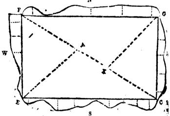
You are supposed to enter the field at C, and as you chain from C to E take up the South off-setts to the left hand—Next chain the second station from E to F, an take up the West off-setts—Chain from F to G, takin up the North off-set—and then chain from G to C, taking up the last off-set—Lastly, measure the Trapezing C E F G, by chaining the base line C F, & take the rig! hand off-sett X G, and the left Y E.
