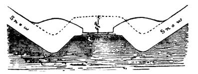
The snow is supposed to be five feet in perpendicular depth, the dotted line shows where its surface would be supposing the Railway to have been closed all winter, and the full line shows where the snow would be deposited along the side, on being cast to the right and left from the rail track.
