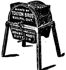
Is the favorite among all Pulpers, having won all the first prizes last year, and a saver of time and labor to the operator, and one which sells at sight after a careful inspection, as it will either pulp coarse or fine, or slice by simply turning over the centre grate and turning crank the reverse way ; and is considered in either capacity superior to any single machines.
