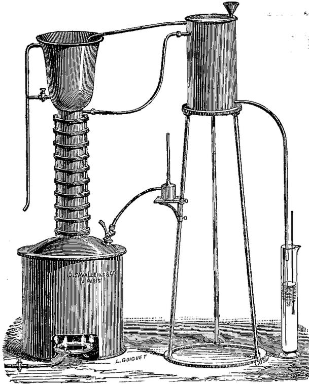
Apparatus of precision for determining the alcoholic
