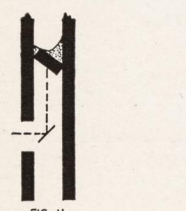
FIG 11 HOW TO USE A MIRROR TO LOOK UP A FLUE.
