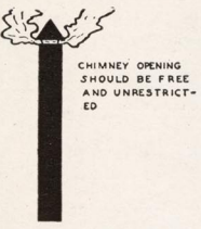
FIG 8 EFFECT OF POORLY DESIGNED FLUE CAP.
